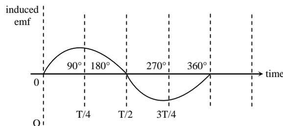
The mechanical energy spent in rotating the coil in magnetic field appears in form of electrical energy.
