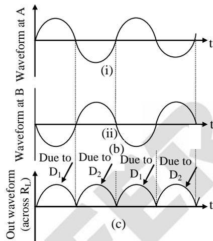
In general full wave rectifier is used to convert AC into DC.
