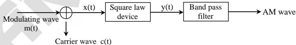
**Fig.** Block diagram for a simple modulator for obtaining an AM signal
