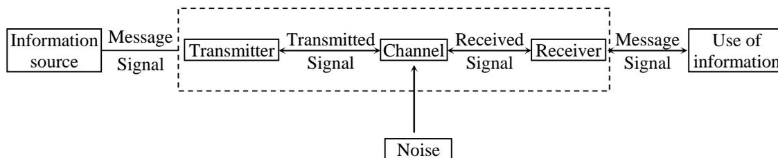
**Transmitter :-** A transmitter is an arrangement that converts the message signal to a form suitable for transmission and then transmits it through some suitable communication channel.
