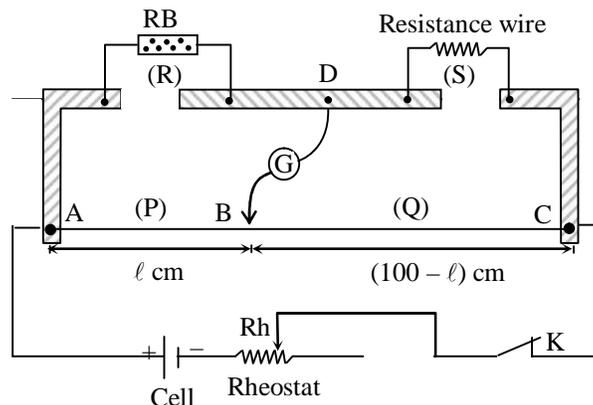
Principle :- It is constructed on the principle of balanced wheatstone bridge.
