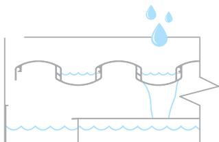
The unique louver profile allows the louvers to interlock, creating the largest rain channels in the industry. Thus, allowing for more water to flow freely into our 360 degree integrated gutter system. StruXure's patented Pass Through Gutter technology allows for rain water to pass from one independent zone to the next allowing for superior drainage performance.
