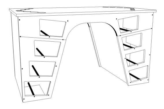
Final Step: Insert plastic trays fully into openings. Your InI is now completely assembled. We recommend labeling the sorting slots in the top with removable labels to assist with sorting.
