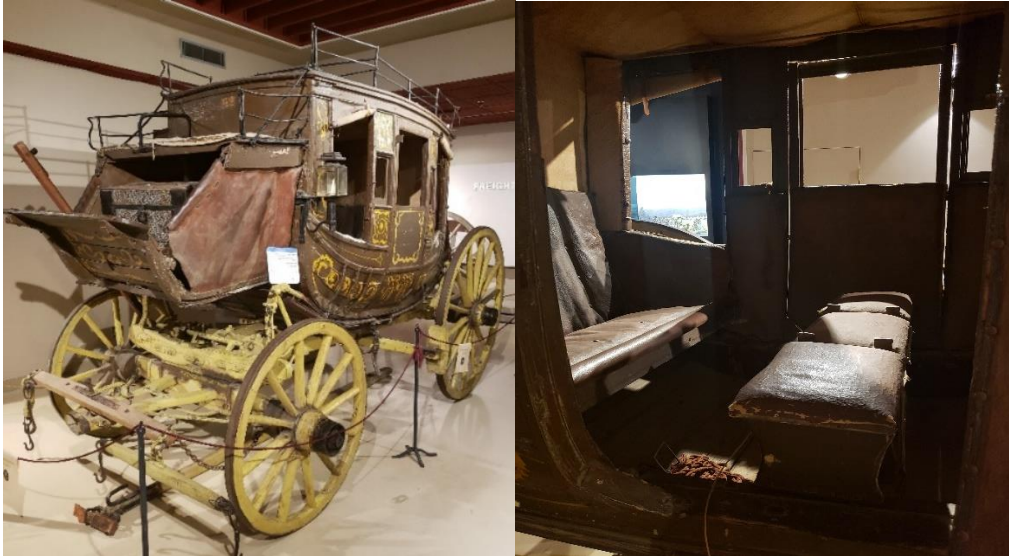
Concord coach exterior and interior, showing one of the sidelights, the rear and middle seats, left-side door, and the raised window in the door (Arizona History Museum, Tucson, author's photograph)
