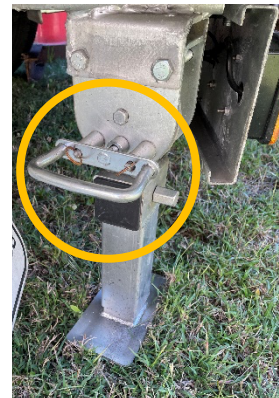
Image 2b: Rear Leg Release Handle Locked in Position
