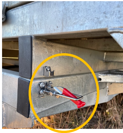
Image 1: Locking Clamps Unclipped
