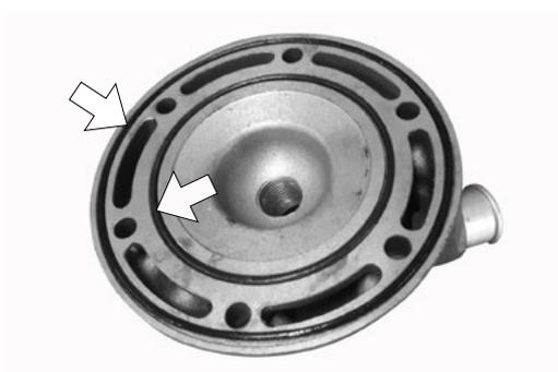
Remove the cylinder head and its O-ring.
