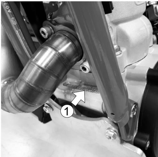
You can identify your specific engine model by means of a code located on the front of the engine below the exhaust elbow, as shown in the image (1).
