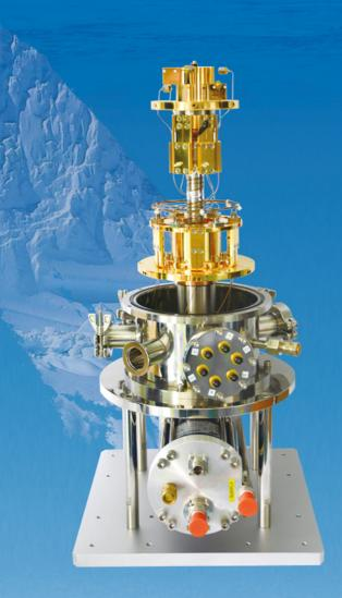
The ultra-low temperature cryostat (Limit temperature < 2.3K) used in superconducting single photon detection system(SNSPD) is a standard and technically mature product of our company, which has been applied in quantum communication successfully. The SNSPD system using this cryostat has an apparent advantage over traditional semiconductor (APD, PMT) detection technology in detection performance (Including detection efficiency and dark count, etc.).
