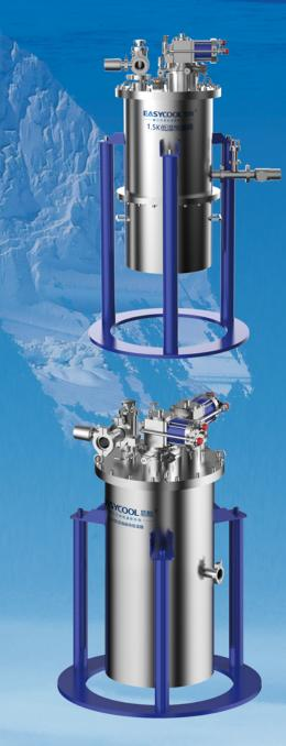
This cryostat takes GM Cryocooler as its cold source and uses JT Throttling technology and Evacuation decompression technique. It can realize <1.5K ultra-low temperature and have a little helium consumption and short cooling down time features.
