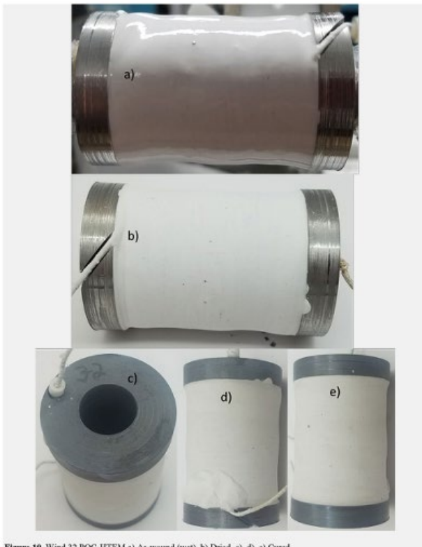
Figure 10. Wind 32 POC-HTEM a) As-wound (wet), b) Dried, c), d), e) Cured
