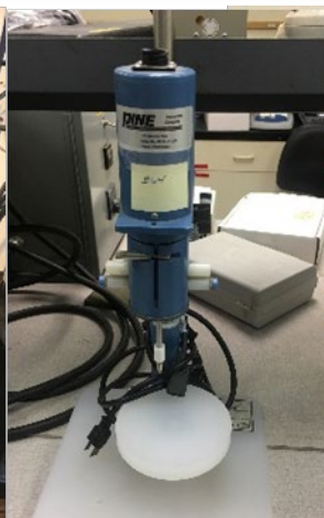
Precision rotator for hydrodynamic modulation of electrodes and optimization of flow conditions
