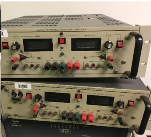
Bipolar power supplies for pulse plating, and current/potential waveform modulation and optimization
