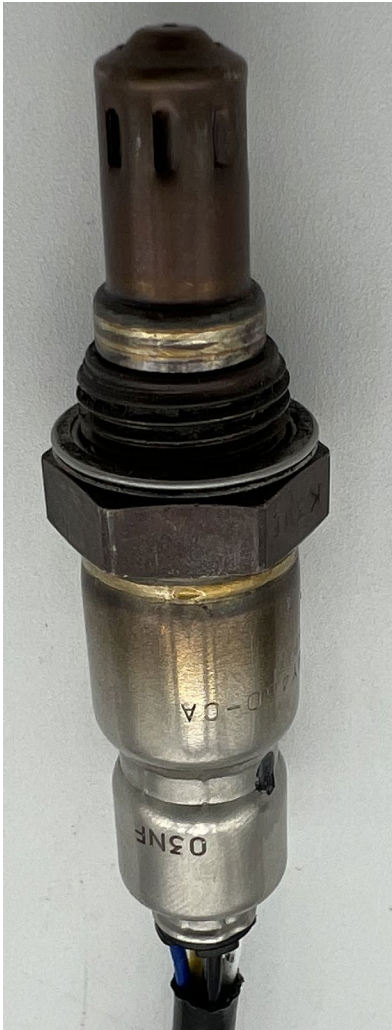
Optical and X-ray Images of 5-Wire Automotive Oxygen Sensor with Integral Heater
