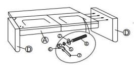
Attach the four part B side legs and two part C middle legs with part 1 Bolt and part 2 flat washers, two bolts/flat washers per leg.
