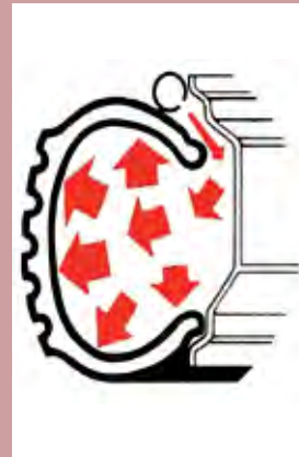
Principle of the Omega Bead Seater
