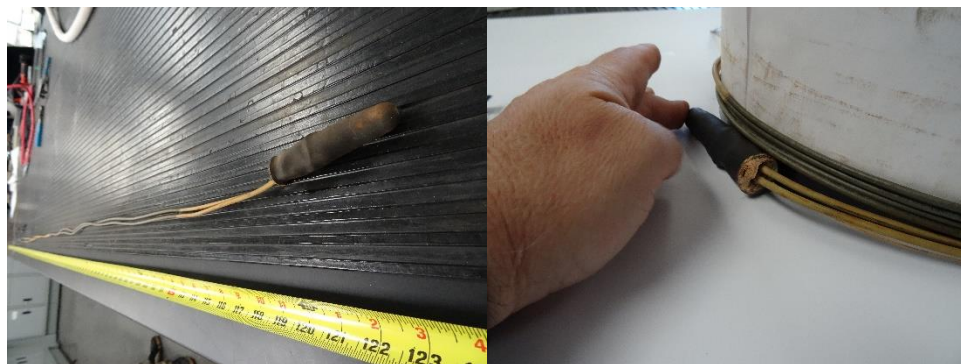
Figure 15: Sample 3 straighten and 20 times bend (basic exposure)
