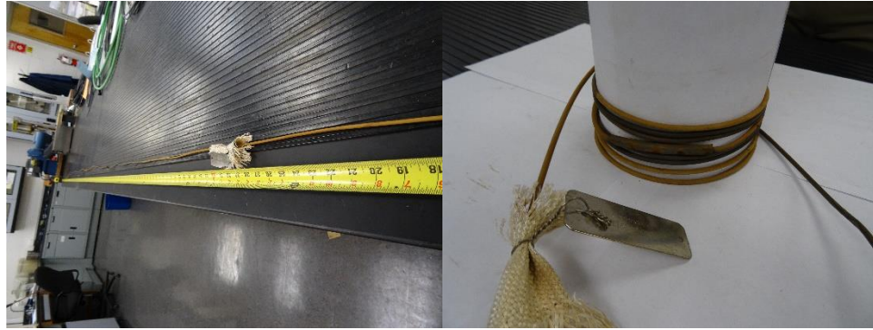
Figure 8: Sample 13 straighten and 20 times bend (acidic exposure)
