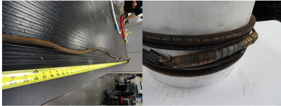
Figure 20: Sample 25 straighten and 20 times bend (basic exposure)
