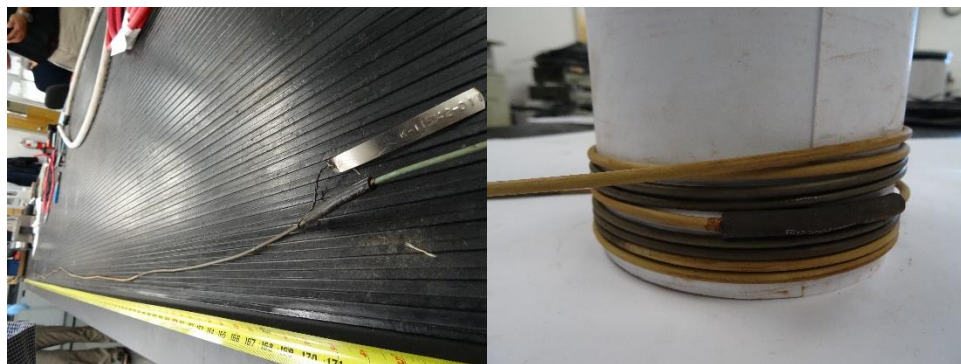
Figure 17: Sample 11 straighten and 20 times bend (basic exposure)
