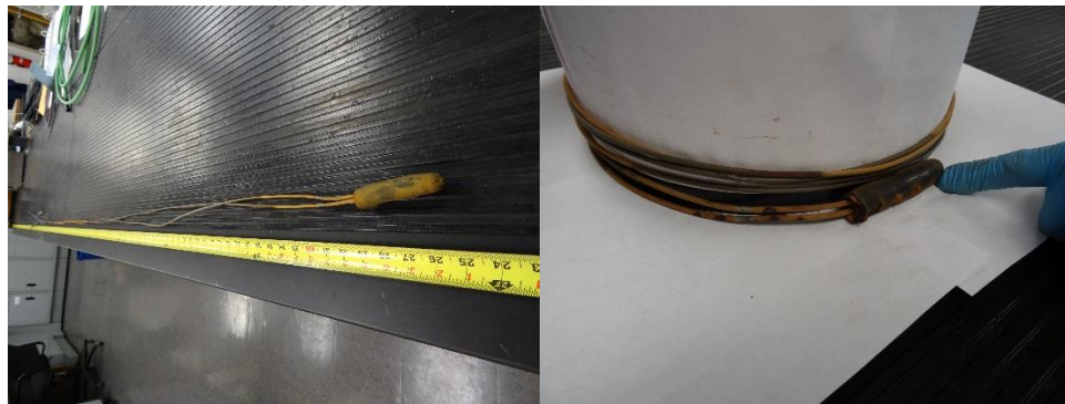
Figure 7: Sample 7 straighten and 20 times bend (acidic exposure)
