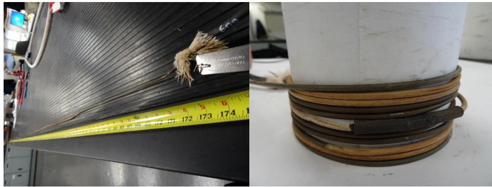
Figure 16: Sample 9 straighten and 20 times bend (basic exposure)
