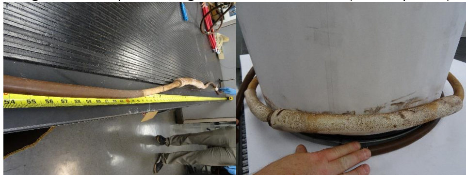
Figure 18: Sample 17 straighten and 20 times bend (basic exposure)
