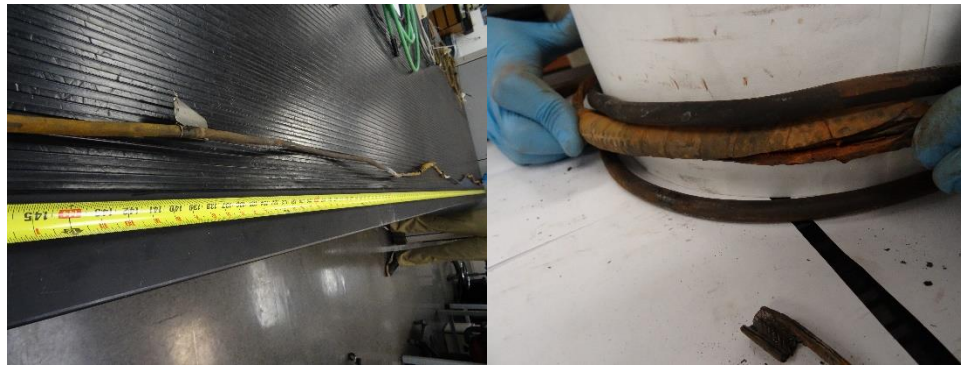
Figure 12: Sample 26 straighten and 20 times bend (acidic exposure)
