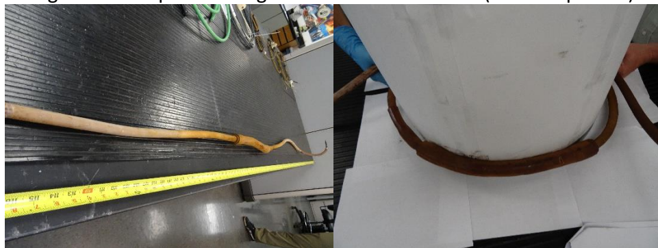
Figure 10: Sample 21 straighten and 20 times bend (acidic exposure)
