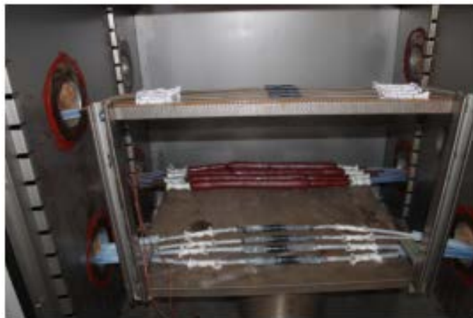
Photo F.6 Overall mounting arrangement for thermal aging Note: Photo taken prior to install of middle shelf used to support V-Type samples.
