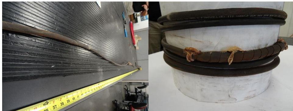
Figure 21: Sample 28 straighten and 20 times bend (basic exposure)
