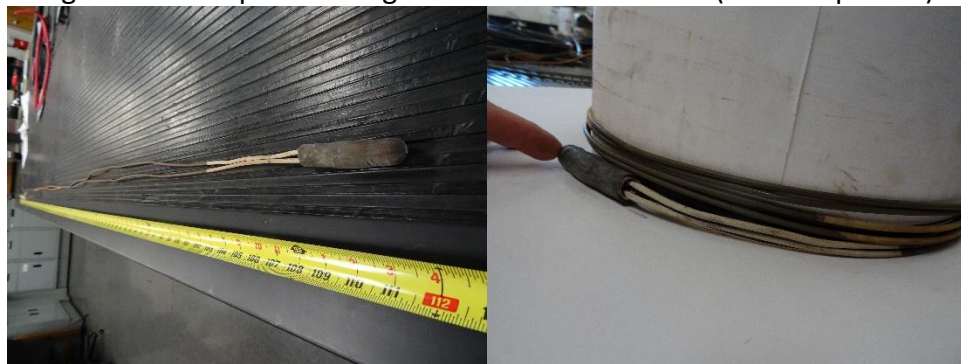
Figure 14: Sample 1 straighten and 20 times bend (basic exposure)
