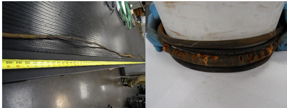
Figure 13: Sample 31 straighten and 20 times bend (acidic exposure)
