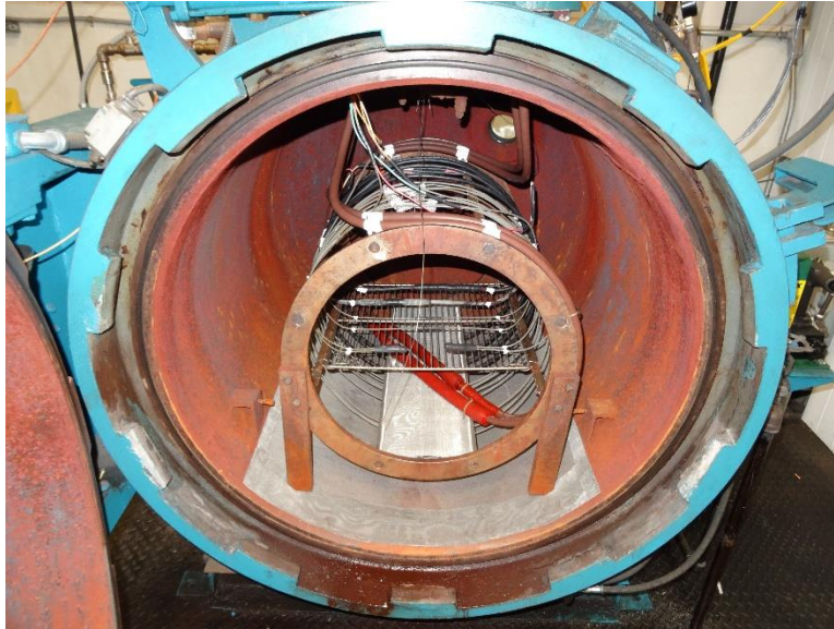
Figure 1: Samples on mandrel prior to acidic environmental exposure
