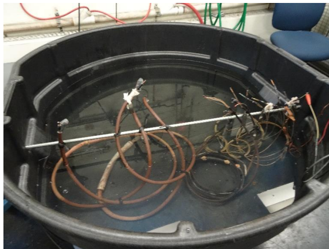
Figure 23: Basic exposure samples submerged
