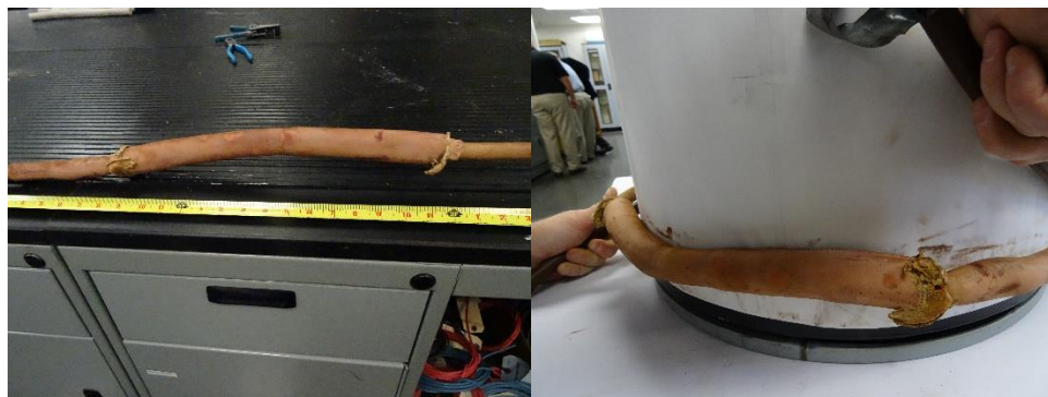
Figure 19: Sample 19 straighten and 20 times bend (basic exposure)
