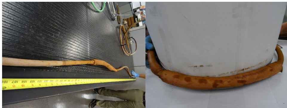
Figure 11: Sample 23 straighten and 20 times bend (acidic exposure)
