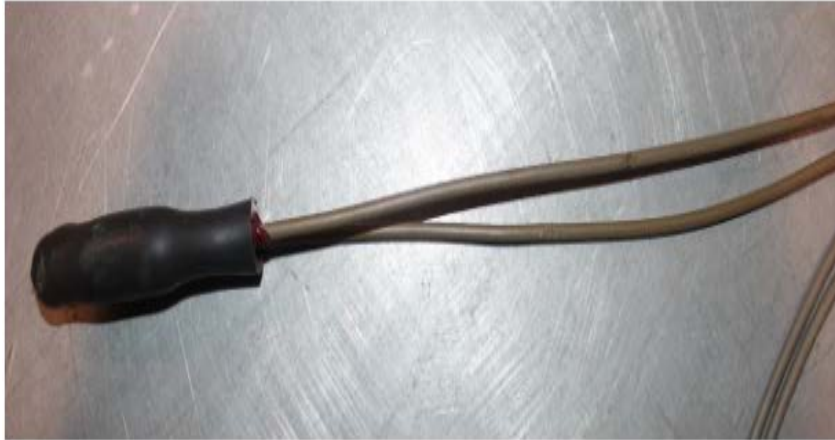
Photo F.1 Typical View of a V-type wire splice sample
