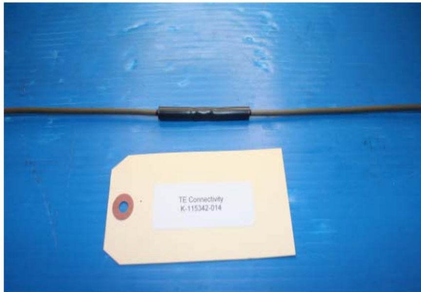
Photo F.2 Typical View of in-line splice sample
