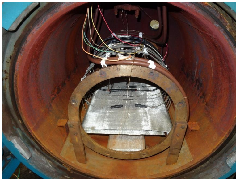
Figure 2: Samples on mandrel prior to basic environmental exposure
