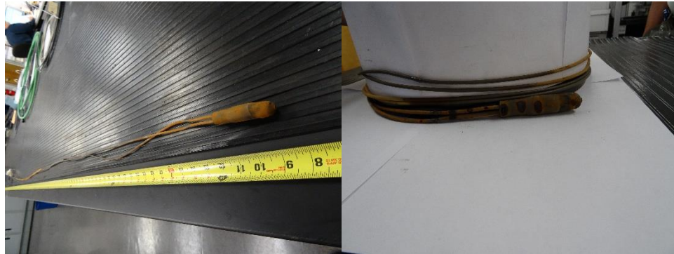
Figure 6: Sample 5 straighten and 20 times bend (acidic exposure)
