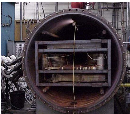
**Figure 9:** LOCA simulation test chamber after the test.
