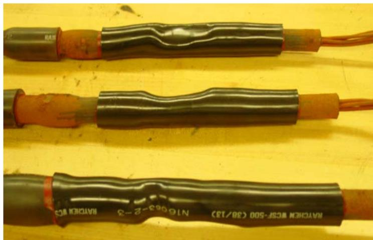
**Figure 14:** Exposed conductors were covered with WCSF tubing.
