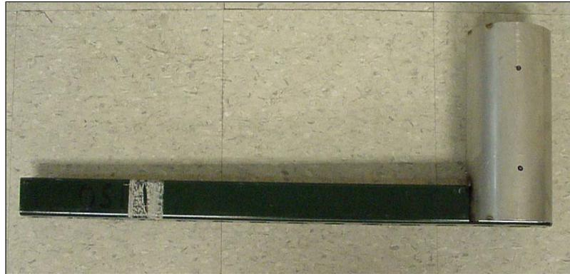
**Figure 1:** Side view of a typical mandrel. Mandrel diameter may vary according to the test description.
