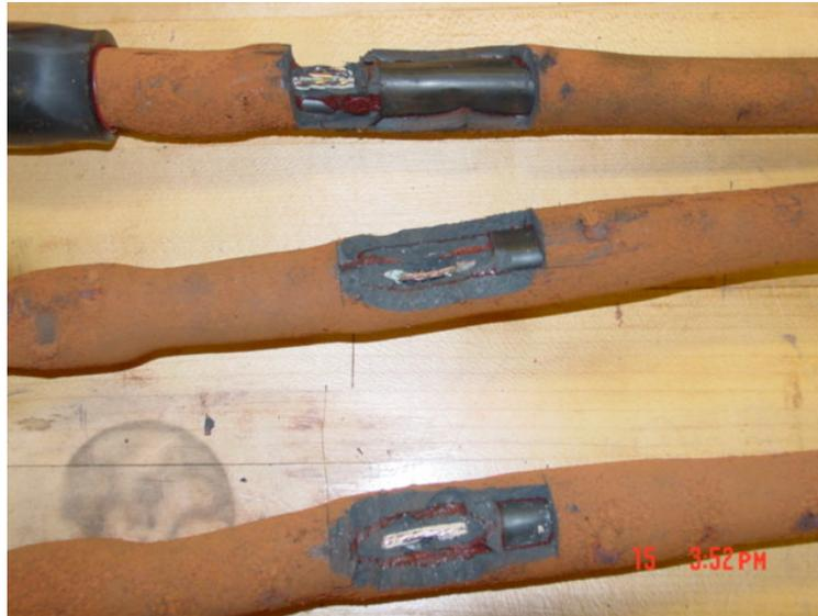
**Figure 13:** Samples were inspected for mechanical integrity and then a single conductor was exposed.
