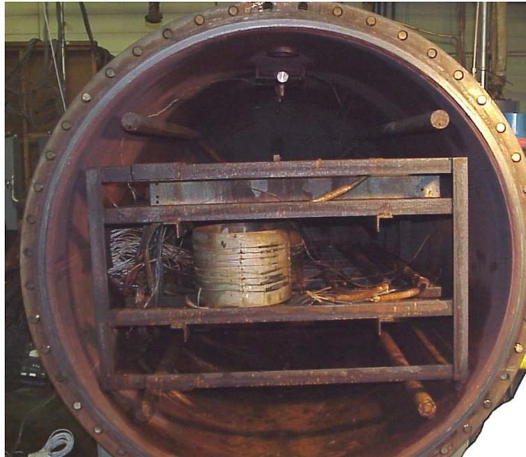
**Figure 8:** LOCA simulation test chamber and internal vessel support frame after the accident simulation.
