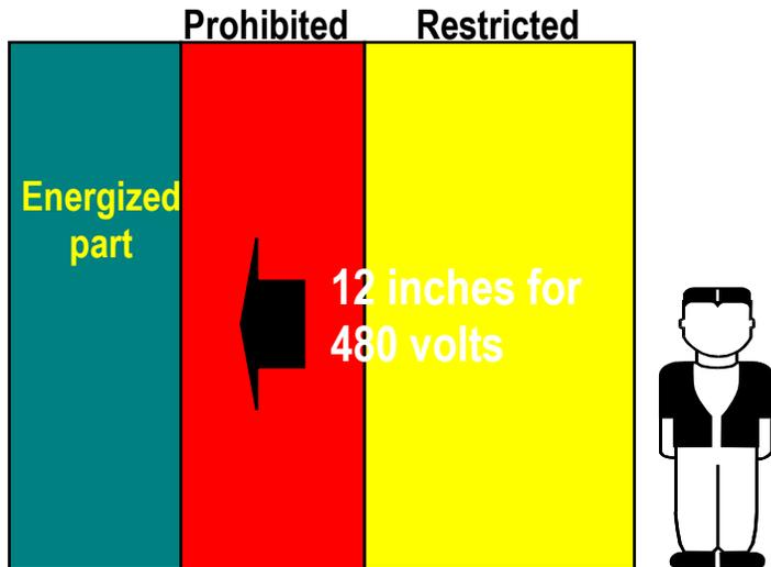
The closest distance to exposed live parts a “qualified” person can approach w/out proper PPE and tools. To cross this boundary, the qualified person must wear PPE and have proper tools.
