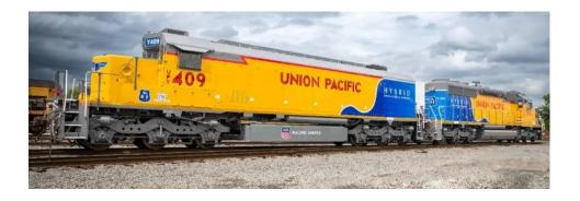
Union Pacific Railroad is testing cutting-edge hybrid battery-electric locomotives designed and bilt by Union Pacific and ZTR. Depending on mode of operation, these hybrid switchers are expected to consume as much as 80% less fuel - reducing associated greenhouse gas and criteria pollutants. Additional benefits include reduced Maintenance expense and noise compared to traditional diesel units.
