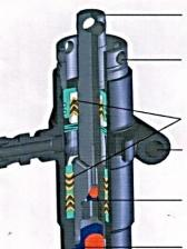
Super hardened, stainless steel piston. Large diameter means fewer cycles per gallon, reducing wear.
