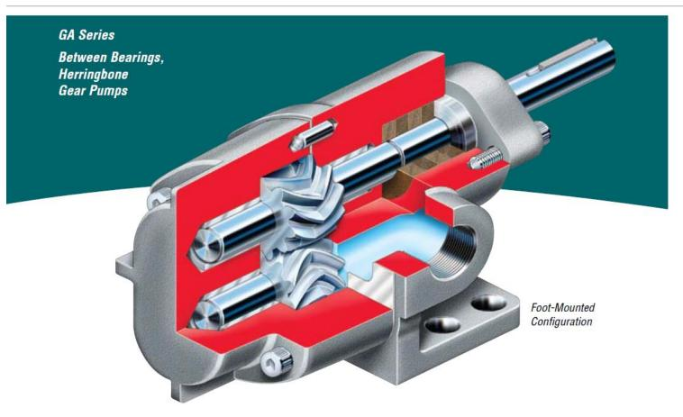
GA Series gear pumps have long been workhorses in highly viscous applications within a multitude of industries due to their dependability, efficiency and low total life cycle costs. Engineered to reliably pump viscous fluids over a broad range of flows and pressures, the GA Series' superior between bearings, external gear design offers the benefits of pulse-free operation, dry-run capability and ease of maintenance.
