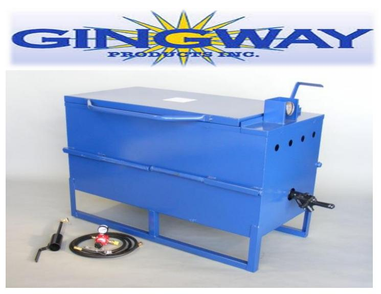
30-Gal Flex Kettle can provide hot material in 30 min or less. It is built with 14 gauge steel. Standard features include temperature gauge with guard, built in hand agitator, lifting handles, and hinged lid. Comes with a 50,000 BTU burner, 10' hose, regulator, striker, and draw-off valve. The kettle is capable of melting up to 1200 lbs. of sealant per day.
