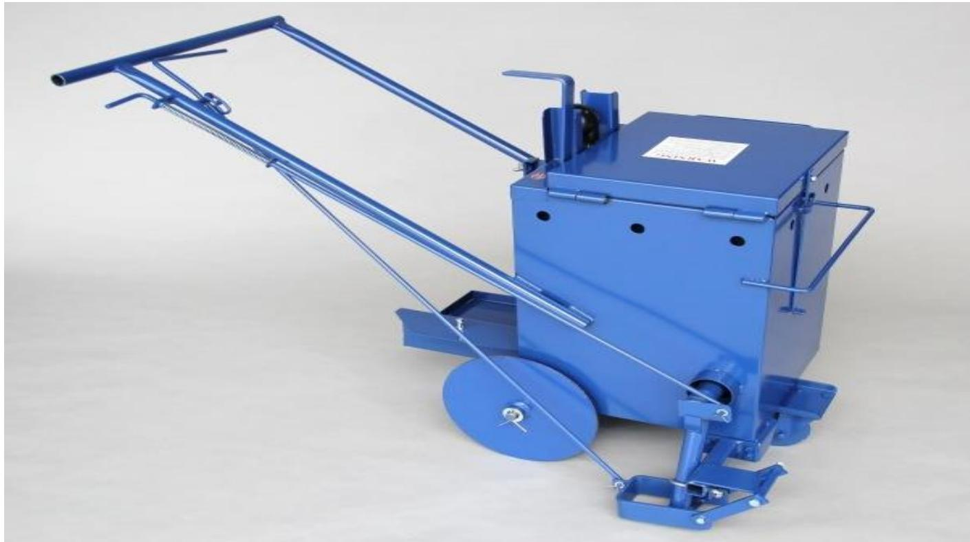
**MA10 Melter/Applicator** is a fast and efficient method for the application of hot applied crack sealants. It can also apply materials from stationary kettles or any large Melter. It can be used without heat for cold pour materials. It is capable of melting and applying 600 lbs. of sealant per day.
