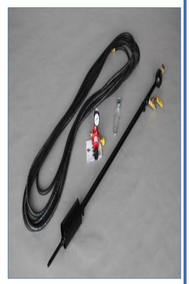
Combined with your air compressor and propane source, the P.A.T. (propane, air, torch) torch will create a high heat output along with a high-speed blast of air to clean and dry cracks in the work area. Made of 3/8" and 1/2" aluminum pipe. comes complete w/ torch, 50' hose, regulator, and striker
