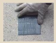
Step 2 after removal of the white wax paper, press the exposed side onto the surface where the reflector is to be located
