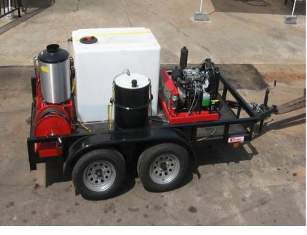
Convenient throttle controls and electric start are standard
