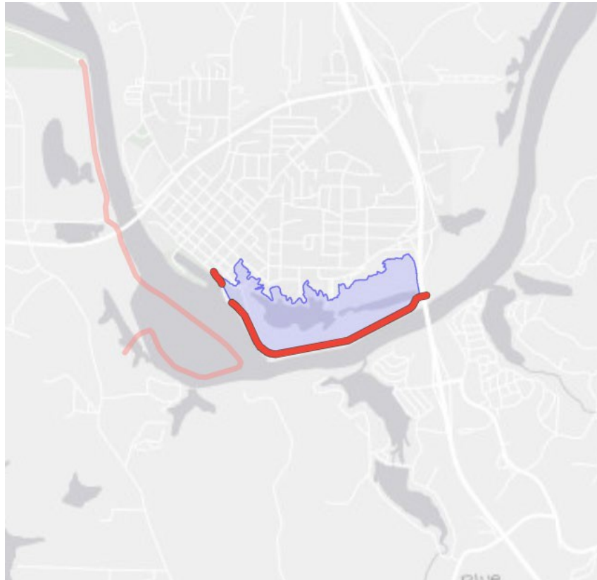
Figure 3.4. County Levees Shown on DFIRM as Providing Protection from the 1-Percent Annual Chance Flood
