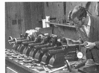
Conover Lathes are hand assembled in small lots. Frequent quality checks during the manufacturing process combined with a dynamic "run in" insure that your lathe is tuned to perfection.
