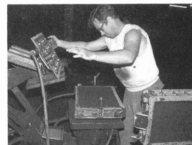
Drag of a flask coming off the squeeze machine and about to go to the foundry floor.
