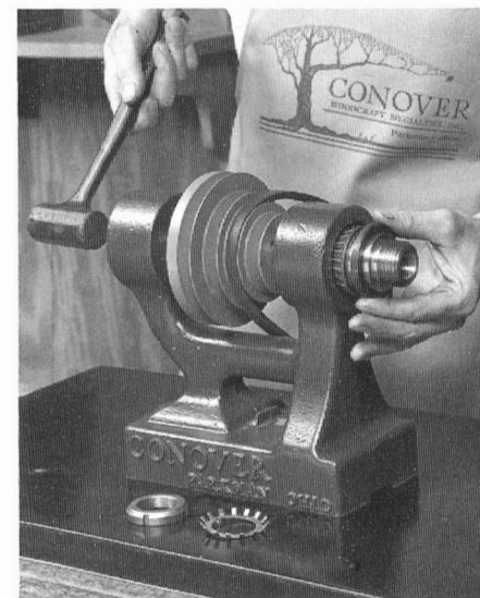
Removal of the headstock spindle. Slight blow from a soft faced mallet coaxies front seal out which technician is now holding.
