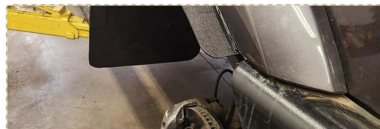
Fenders trimmed to clear the larger off-road tires
