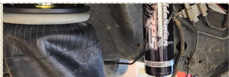
Air suspension and adjustable shocks
