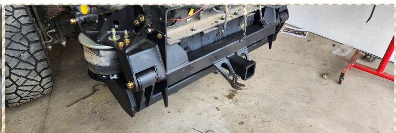
The Kelderman system: leaf spring hanger replaced with an airbag
