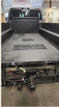
The three access panels: both fuel pump modules, and the open middle slot for a future gooseneck
