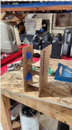
Cardboard mockup for the fuel filler angles
