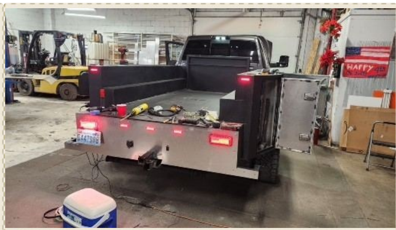
The completed taillight panel, plate and all
