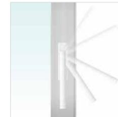
Moving the handle 180° actually lifts the operating panel off the sill, enabling it to glide effortlessly.
