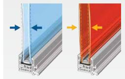
With conventional aluminum spacers, the sealant flexes, which can lead to sealant failure and loss of insulation performance.
