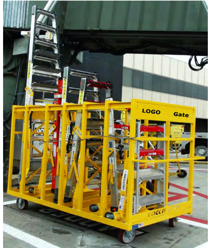
The LockNCart2 allows easy storage of line ladders corresponding to color-coded system.
