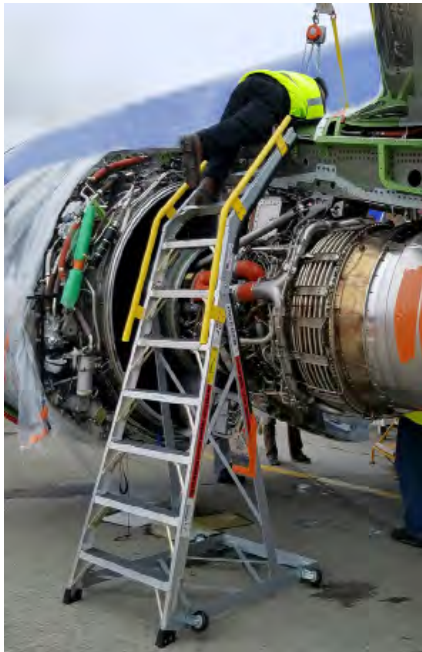
Boeing 737: Ladder confirms to engine profile and allows technician comfortable prone working access.
