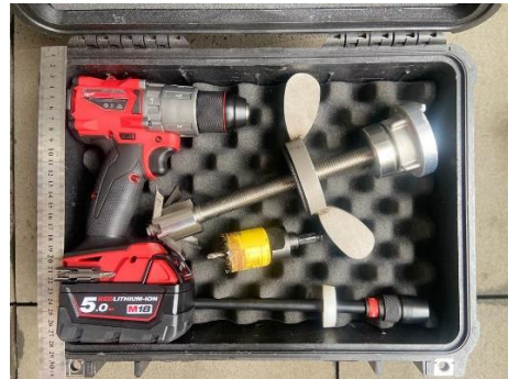
Figure 9: 316-grade Stainless Steel BAT prototype to suit 3/8-inch nozzle (nozzle not included) with drilling equipment in portable shockproof case.
