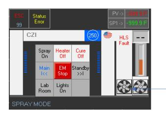
Hold the Left Blower for 4 seconds to get the VFD display
