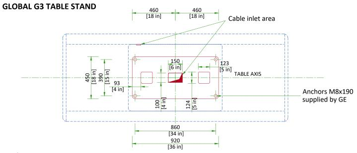
The floor bearing the system is recommended to be concrete and the thickness to be determined by a Structural Engineer to properly support the equipment loads. The supplied anchors require a minimum embedment of 90 mm [3.5 in] into the concrete. If the floor thickness is less than 95 mm [3.7 in], it is recommended that the unit be secured using a through-bolt method with a reinforcement plate on the back side.
