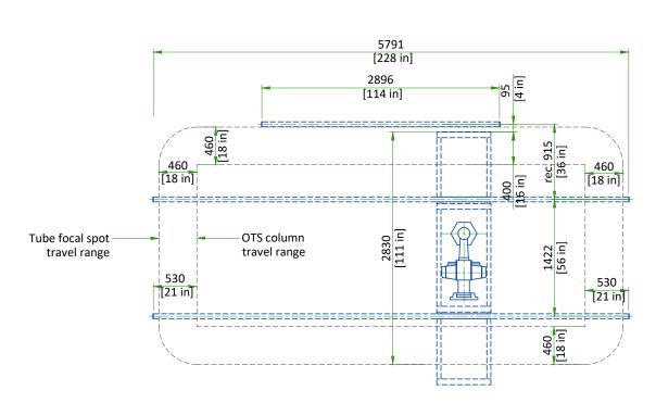
Note: Focal Spot Travel depends on the length of the bridge, rails and position of bridge. NOT TO SCALE
