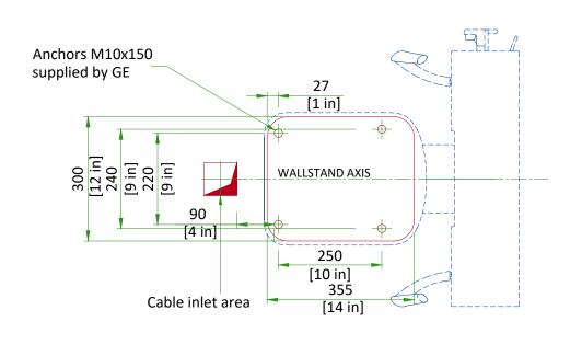
Concrete area for wall stand installation should be 1 m<sup>2</sup> [39.37 ft<sup>2</sup>].
