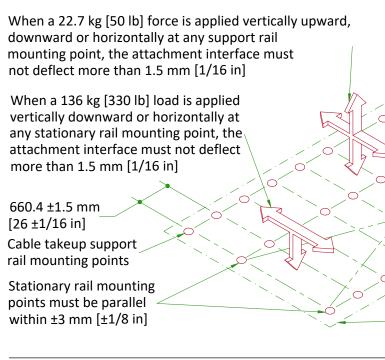
Distance between holes axis 660.4 mm [26 in], Maximum load per screw is 160 kg [353 lb], however each mounting screw must not "PULL OUT" or otherwise fail under a vertically downward dead load of 635 kg [1400 lb]. Bolts for mounting stationary rails on Unistrut or equivalent supplied by GE (1/2" - 13) headed bolts)
