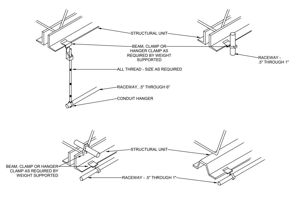
1 TYPICAL RACEWAY SUPPORT METHODS DETAIL SCALE: NTS
