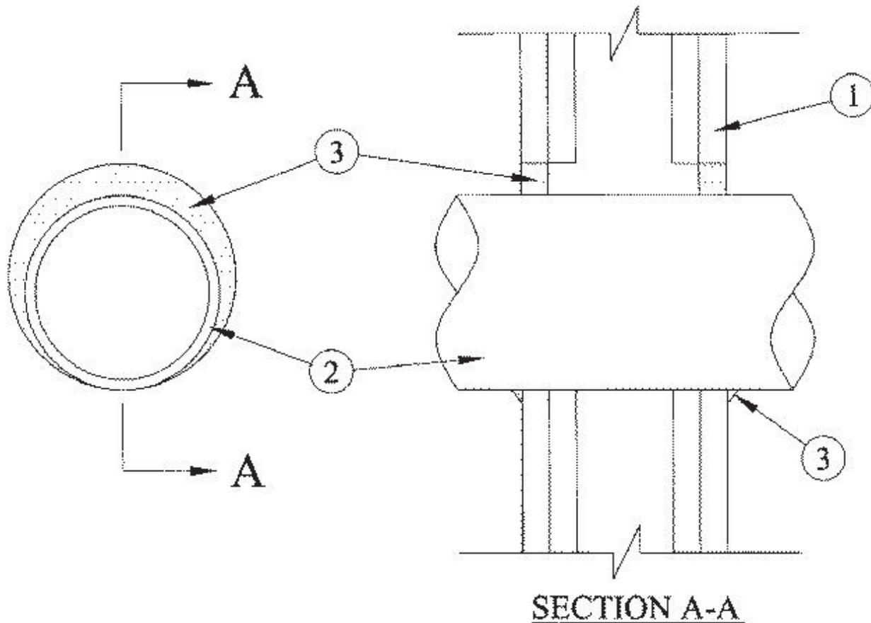
**1. Wall Assembly** — The 1 or 2 hr fire rated wallboard/stud wall assembly shall be constructed of the materials and in the manner specified in the individual U300 or U400 Series Wall and Partition Designs in the UL Fire Resistance Directory and shall include the following construction features.
