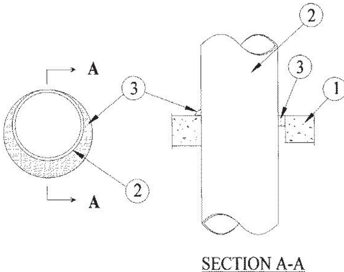
1. **Floor or Wall assembly** — Minimum 4-1/2 in. (114 mm) thick reinforced lightweight or normal weight (100-150 pcf or 1600-2400 kg/m<sup>3</sup>) concrete. Wall may also be constructed of any UL Classified **Concrete Blocks\***. Maximum diameter of opening is 30-7/8 in. (784 mm).
