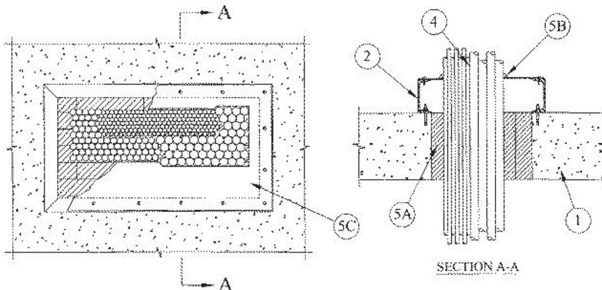
1. **Floor or Wall Assembly** — Min 8 in. (203 mm) thick reinforced lightweight or normal weight (100-150 pcf or 1600-2400 kg/m<sup>3</sup>) concrete. Max area of opening is 288 sq in. (1858 cm<sup>2</sup>) with max dimension of 24 in. (610 mm).
