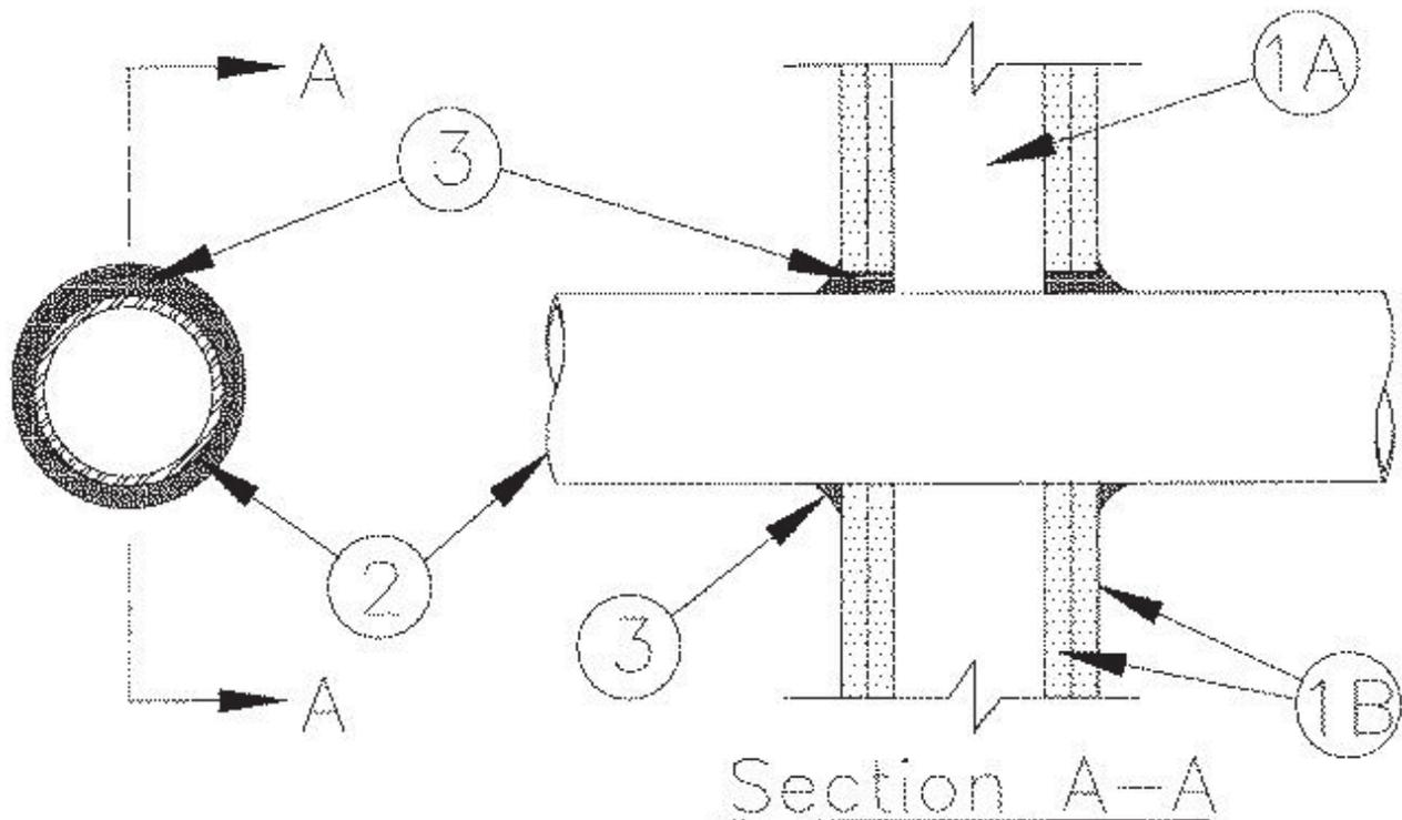
**1. Wall Assembly** — The 1 or 2 hr fire-rated gypsum wallboard/stud wall assembly shall be constructed of the materials and in the manner specified in the individual U300 or U400 Series Wall and Partition Designs in the UL Fire Resistance Directory and shall include the following construction features:
