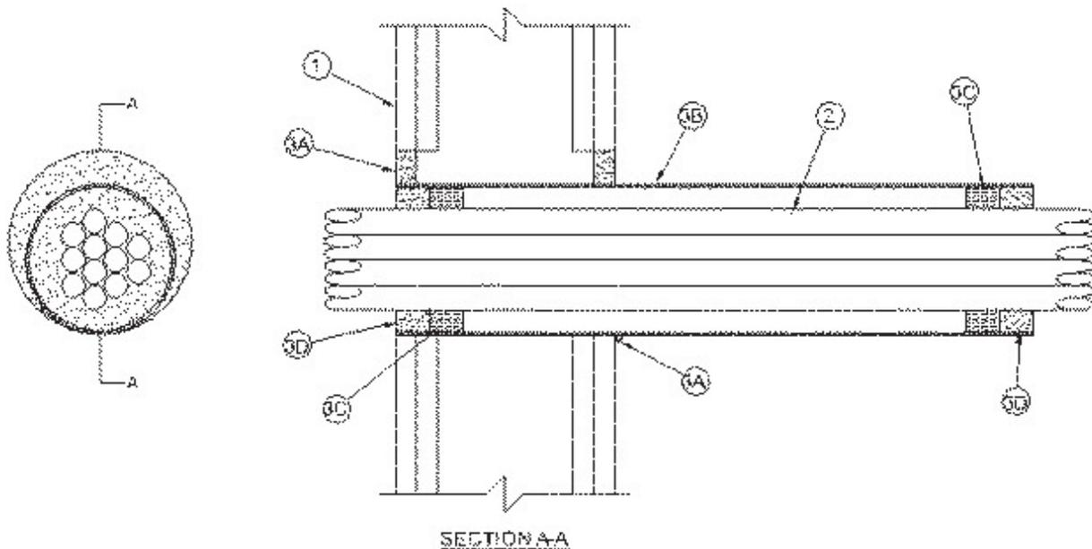
1. **Wall Assembly** — The 1 or 2 hr fire rated gypsum board/stud wall assembly shall be constructed of the materials
