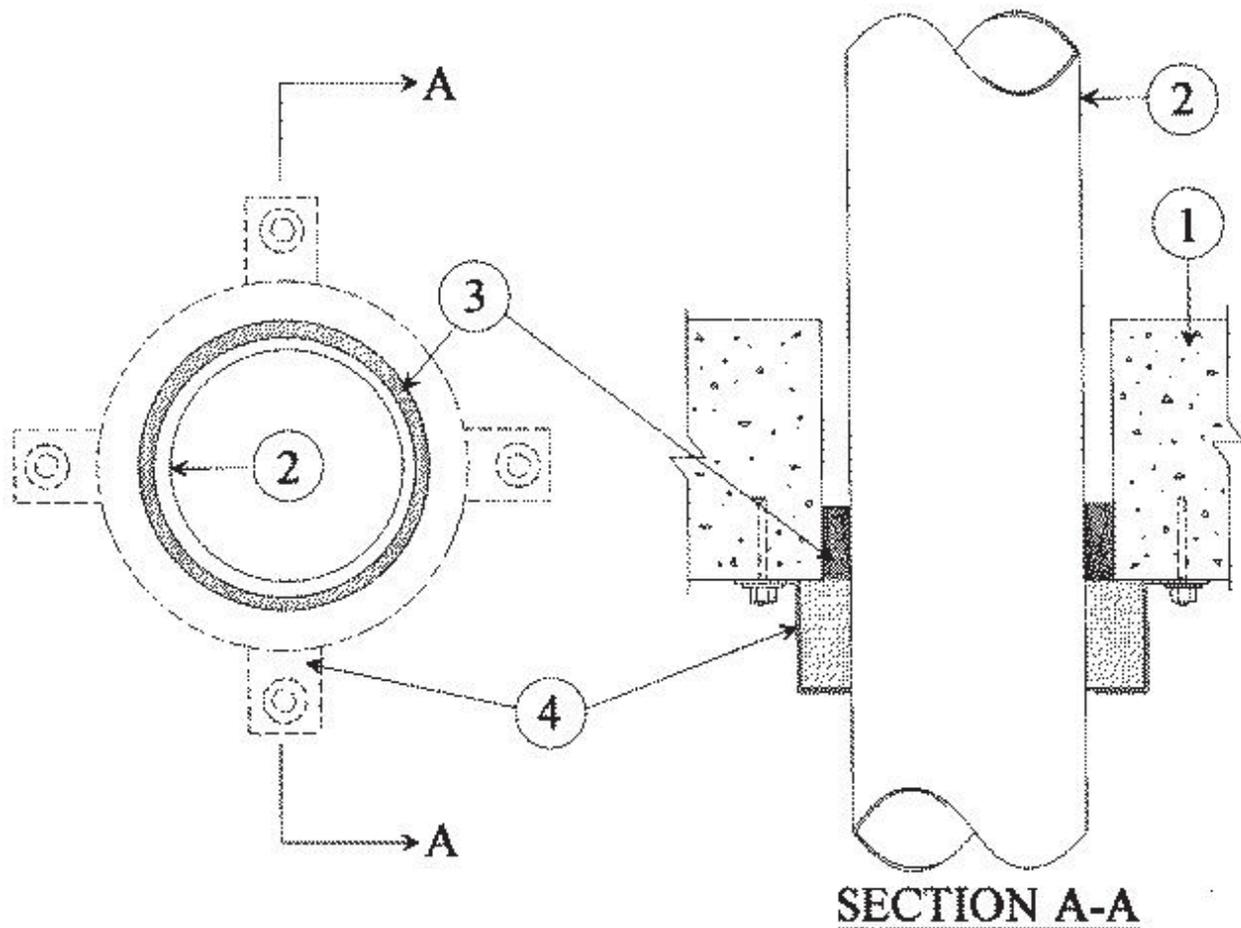
1. **Floor or Wall Assembly** — Min. 4-1/2 in. (114 mm) thick reinforced lightweight or normal weight (100-150 pcf or 1600-2400 kg/m<sup>3</sup>) concrete. Wall may also be constructed of any UL Classified **Concrete Blocks**. Max diam of opening is 7 in. (178 mm).
