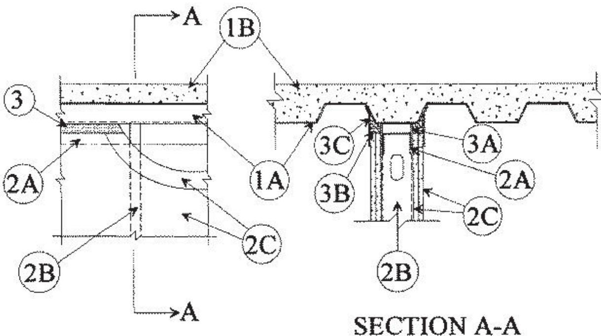
1. **Floor Assembly** — The fire-rated fluted steel deck/concrete floor assembly shall be constructed of the materials and in the manner described in the individual D700 or D900 Series Floor-Ceiling Design in the UL Fire Resistance Directory and shall include the following construction features:
