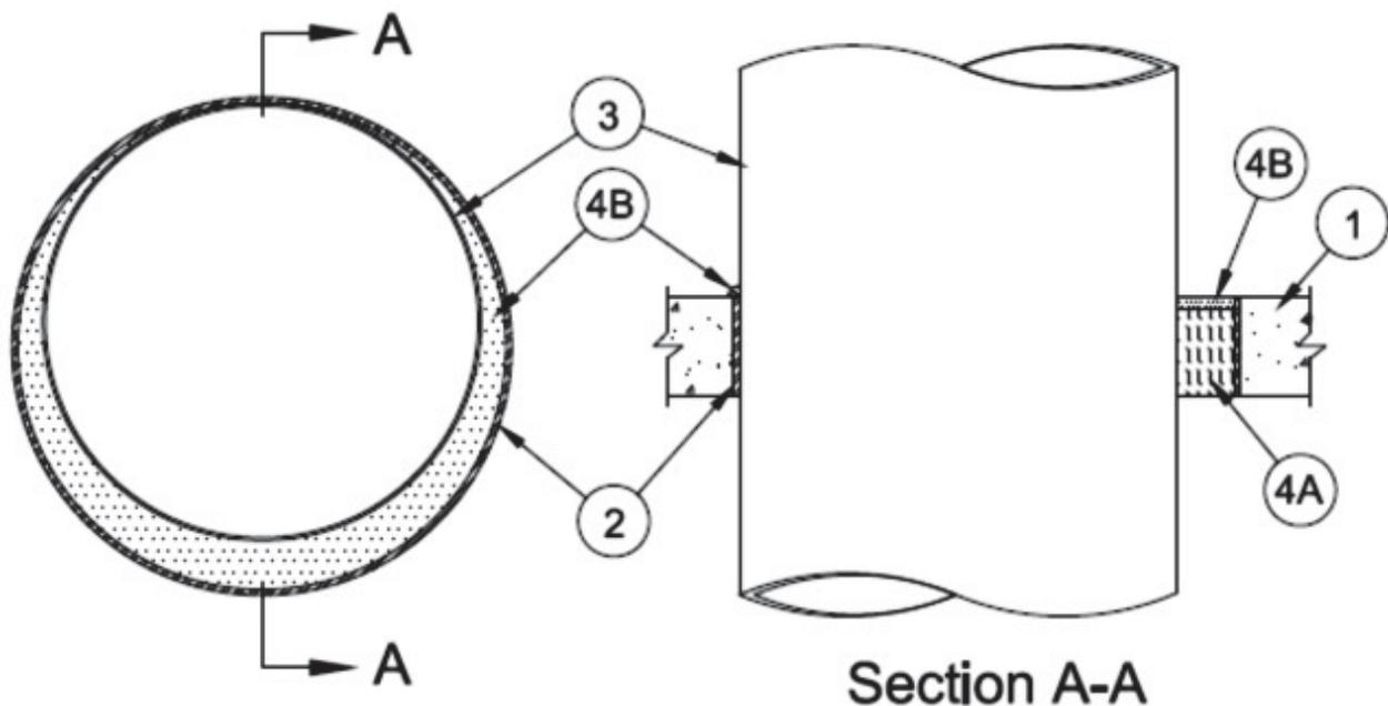
1. **Floor or Wall Assembly** — Min 4-1/2 in. (114 mm) thick reinforced lightweight or normal weight (100-150 pcf or 1600-2400 kg/m<sup>3</sup>) concrete. Wall may also be constructed of any UL Classified **Concrete Blocks\***. Max diam of opening is 32 in. (813 mm).
