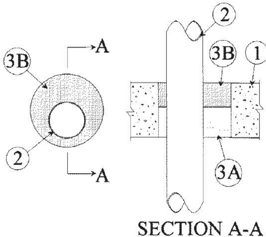
1. **Floor or Wall Assembly** — Min 4-1/2 in. (114 mm) thick reinforced lightweight or normal weight (100-150 pcf or 1600-2400 kg/m<sup>3</sup>) concrete. Wall may also be constructed of any UL Classified Concrete Blocks\*. Max diam of opening is 6 in. (152 mm).
