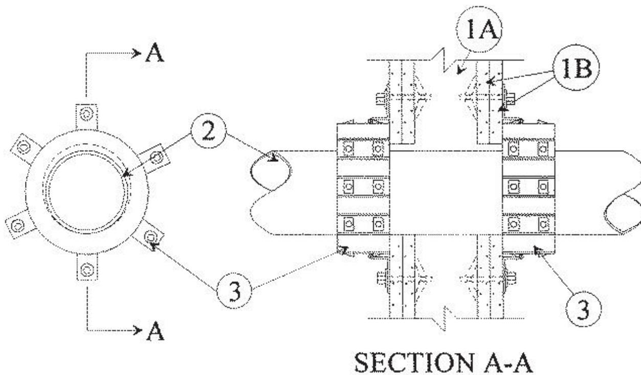
**1. Wall Assembly** — The fire-rated gypsum board/stud wall assembly shall be constructed of the materials and in the manner specified in the individual U300, U400, V400 or W400 Series Wall and Partition Designs in the UL fire Resistance
