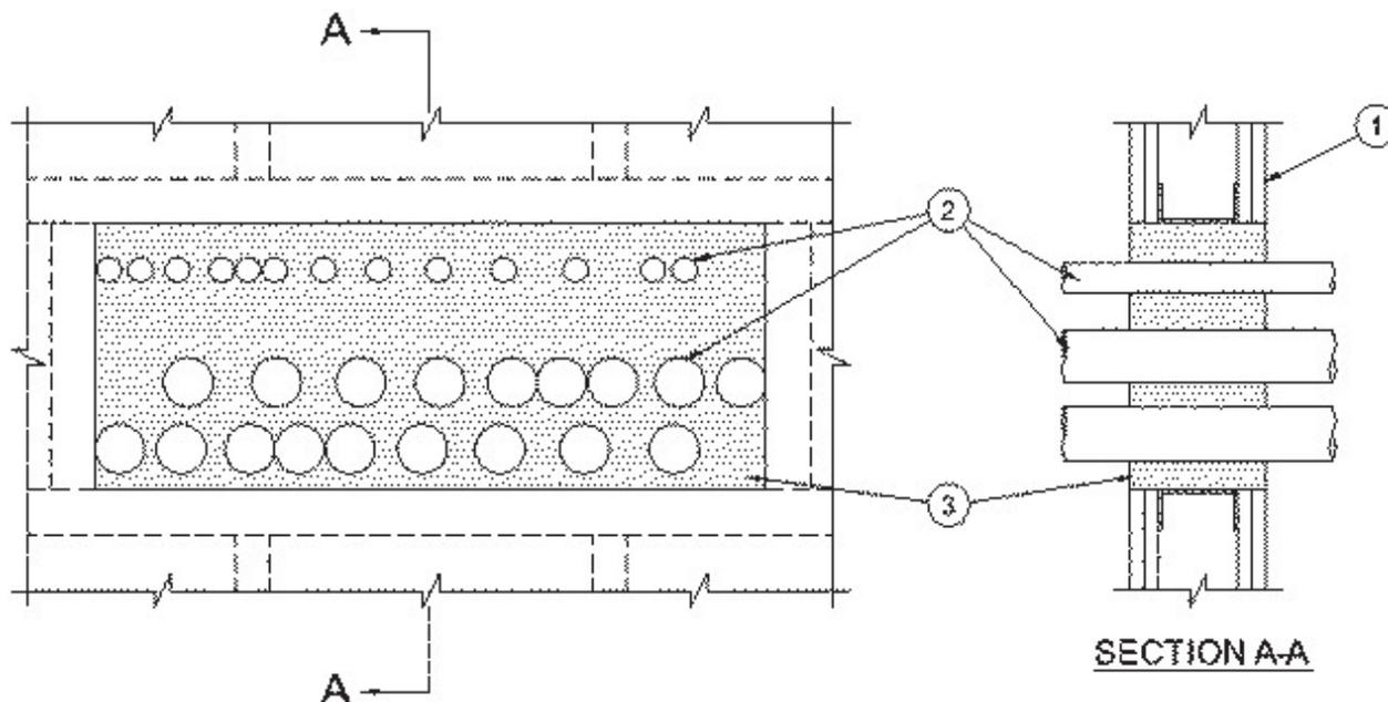
**1. Wall Assembly** — The 1 or 2 hr fire-rated gypsum board/stud wall assembly shall be constructed of the materials and in the manner described in the individual U400 Series Wall or Partition Design in the UL Fire Resistance Directory and shall include the following construction features.
