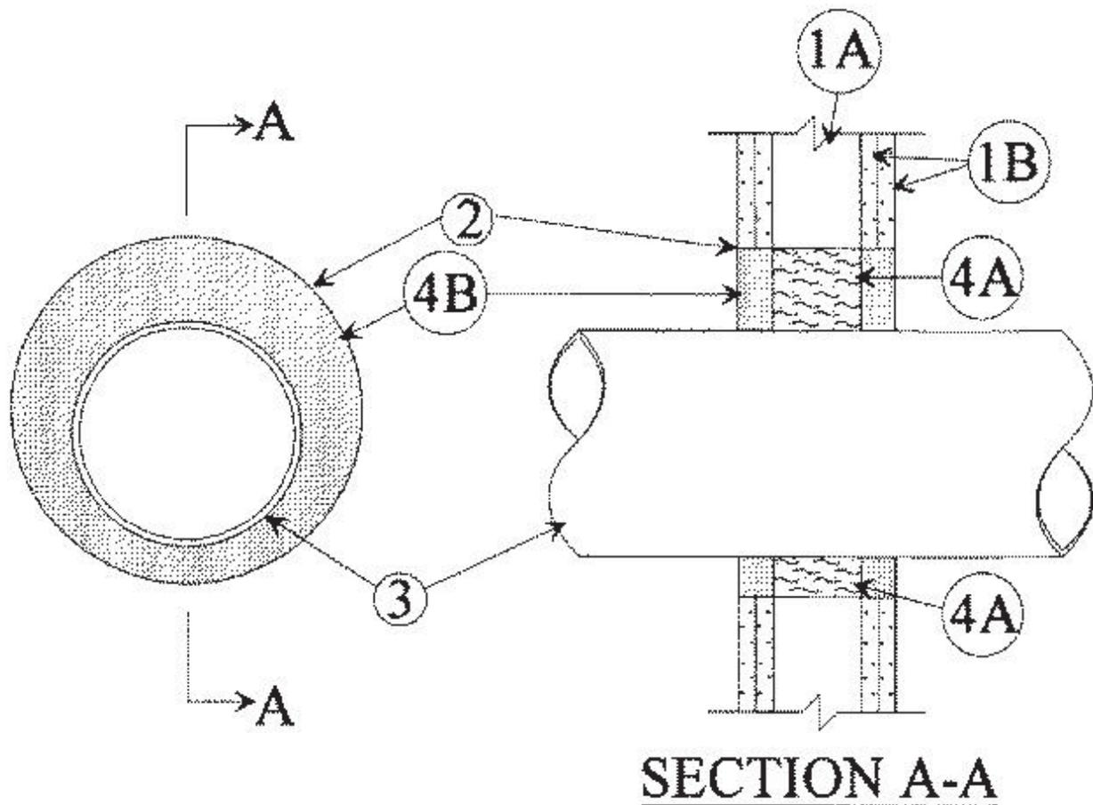
**1. Wall Assembly** — The 1 or 2 hr fire-rated gypsum wallboard/stud wall assembly shall be constructed of the materials and in the manner specified in the individual U300, U400 or V400 Series Wall and Partition Designs in the UL Fire Resistance Directory and shall include the following construction features:
