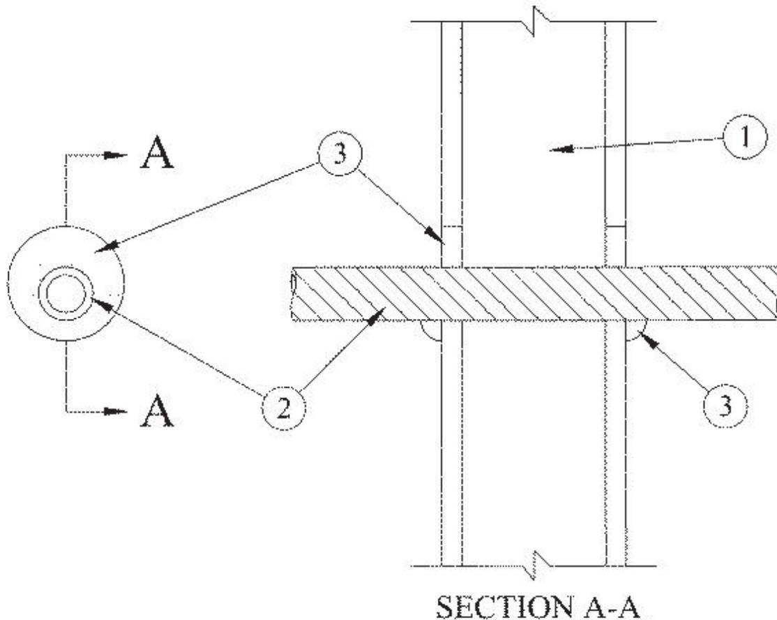
1. **Wall Assembly** — The fire-rated gypsum wallboard/stud wall assembly shall be constructed of the materials and in the manner specified in the individual U300, U400, V400 or W400 Series Wall and Partition Designs in the Fire Resistance Directory and shall include the following construction features:
