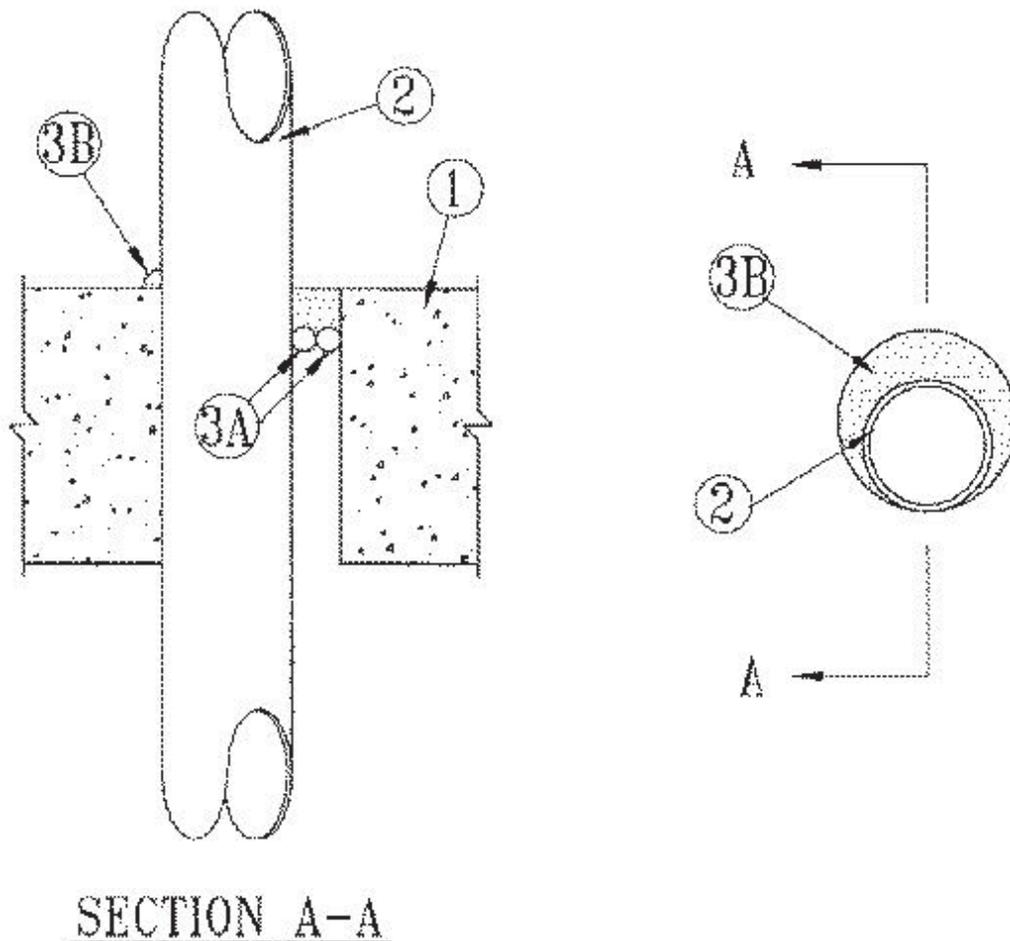
1. **Floor or Wall Assembly** — Min 4-1/2 in. (114 mm) thick reinforced lightweight or normal weight (100-150 pcf or 1600-2400 kg/m<sup>3</sup>) concrete. Wall may also be constructed of any UL Classified **Concrete Blocks\***. Max diam of opening is 4 in. (102 mm).
