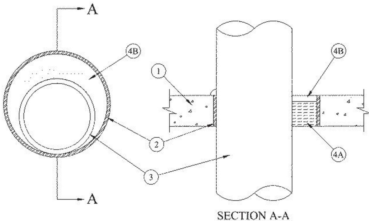
**1. Floor Assembly** — Min 2-1/2 in. (64 mm) thick reinforced lightweight or normal weight (100-150 pcf or 1600-2400 kg/m<sup>3</sup>) concrete. Max diameter of opening is 31-7/8 in. (810 mm).
