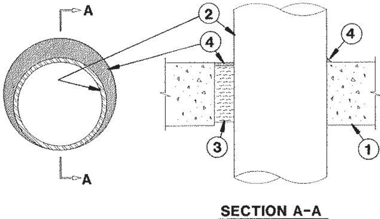
**1. Floor or Wall Assembly** — Min 4-1/2 in. (114 mm) thick reinforced lightweight or normal weight (100-150 pcf or 1600-2400 kg/m<sup>3</sup>) concrete. Wall may also be constructed of any UL Classified **Concrete Blocks** \*. Max diam of opening is 12 in. (305 mm).
