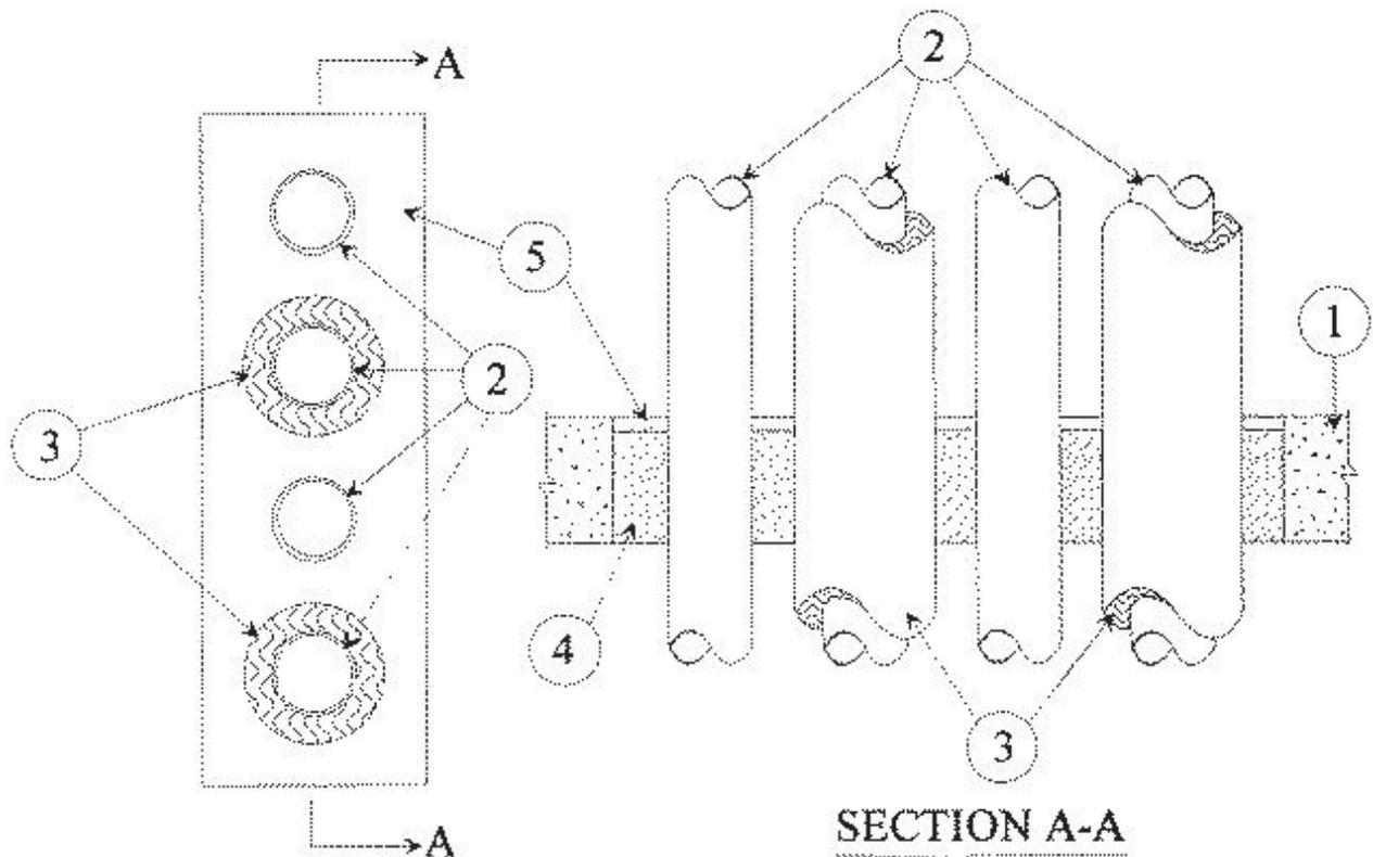
**1. Floor or Wall Assembly** — Min 4-1/2 in. (114 mm) thick reinforced lightweight or normal weight (100-150 pcf or 1600-2400 kg/m<sup>3</sup>) concrete floor or min 5 in. (127 mm) thick reinforced lightweight or normal weight (100-150 pcf or 1600-2400 kg/m<sup>3</sup>) concrete wall. Wall may also be constructed of any UL Classified **Concrete Blocks\***. Max area of opening is 192 sq in. (1239 cm<sup>2</sup>) with max dimension of 24 in. 9610 mm).
