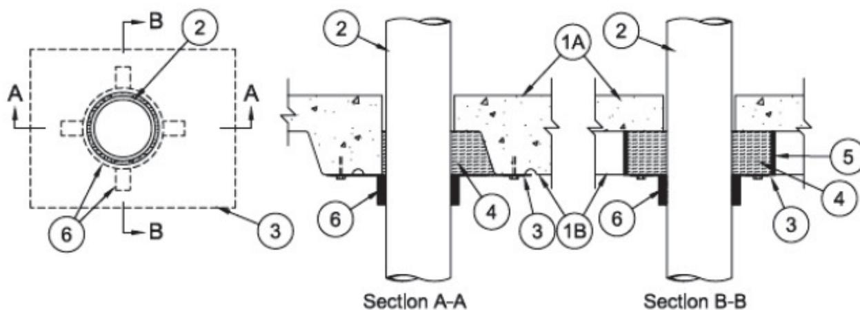
**1. Floor Assembly** — The fire-rated unprotected concrete and steel floor assembly shall be constructed of the materials and in the manner specified in the individual D900 Series designs in the UL Fire Resistance Directory and as summarized below:
