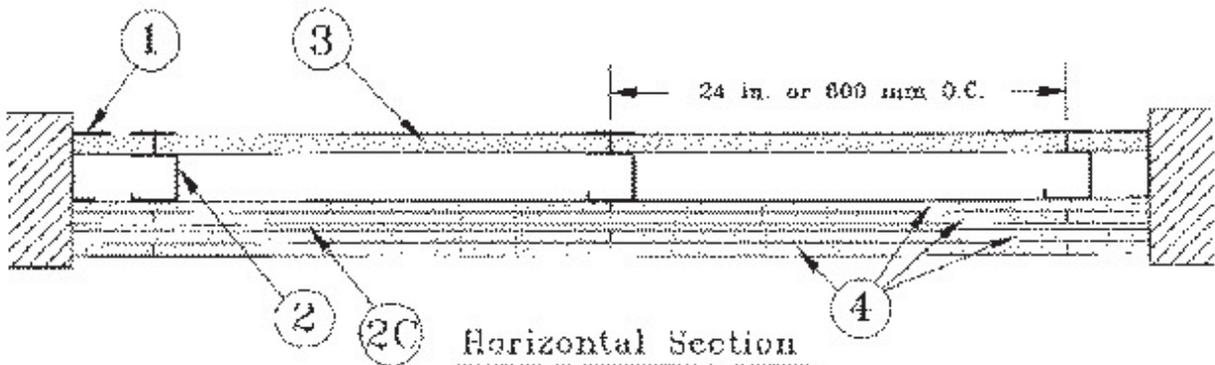
1. **Floor, Side and Ceiling Runners** - "J" - shaped runner, min 2-1/2 in. deep (min 4 in. deep when System C is used), with unequal legs of 1 in. and 2 in., fabricated from min 24 MSG (min 20 MSG when Item 4A, 4B or 7 are used) galv steel. Runners positioned with short leg toward finished side of wall. Runners attached to structural supports with
