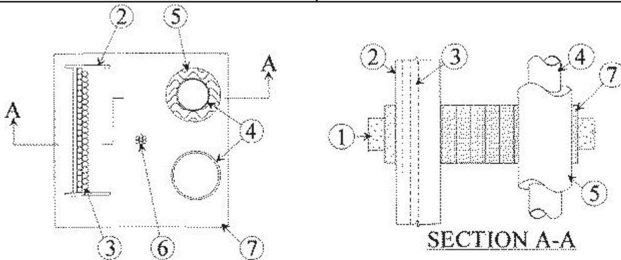
1. **Floor or Wall Assembly** — 4-1/2 in. (114 mm) thick reinforced lightweight or normal weight (100-150 pcf or 1600-2400 kg/m<sup>3</sup>) concrete. Wall may also be constructed of any UL Classified **Concrete Blocks**\*. Max area of opening is
