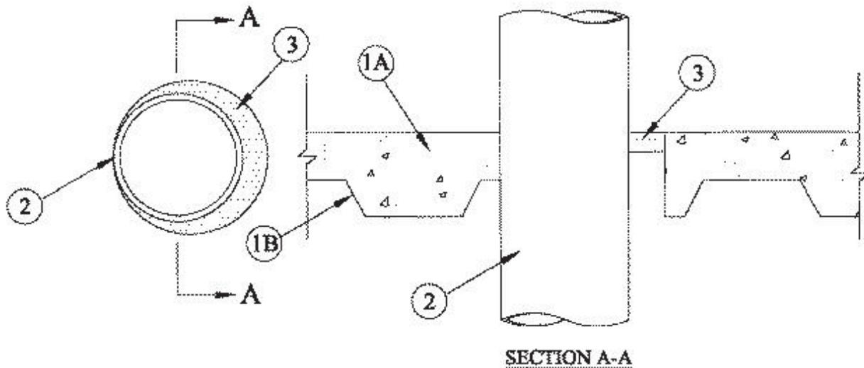
**1. Floor Assembly** — The fire rated unprotected concrete and steel floor assembly shall be constructed of the materials and in the manner specified in the individual D900 Series designs in the UL Fire Resistance Directory and as summarized below:
