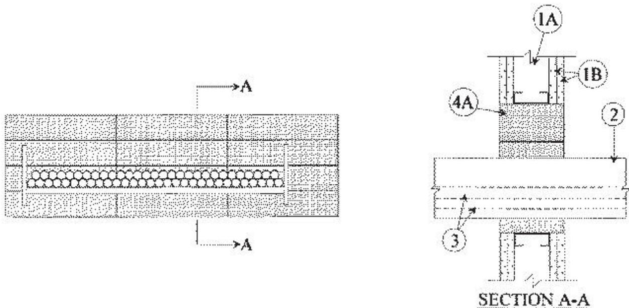
1. **Wall Assembly** — The 1 or 2 hr fire rated gypsum board/stud wall assembly shall be constructed of the materials and in the manner described in the individual U300, U400, V400 or W400 Series Wall and Partition Designs in the UL Fire Resistance Directory and shall include the following construction features:
