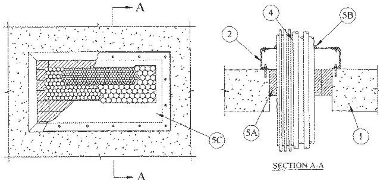
1. **Floor or Wall Assembly** — Min 8 in. (203 mm) thick reinforced lightweight or normal weight (100-150 pcf) concrete. Max area of opening is 288 sq in. (1858 cm<sup>2</sup>) with max dimension of 24 in. (610 mm).
