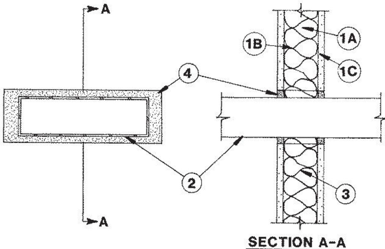
**1. Wall Assembly** — The fire-rated gypsum wallboard/stud wall assembly shall be constructed of the materials and in the manner described in the individual U300 or U400 Series Wall and Partition Designs in the UL Fire Resistance Directory and shall include the following construction features:
