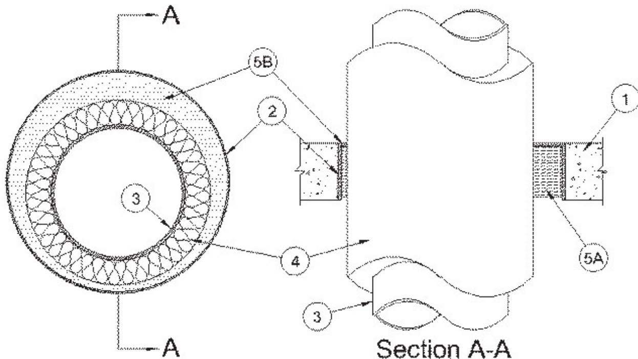
**1. Floor or Wall Assembly** — Min 4-1/2 in. (114 mm) thick reinforced lightweight or normal weight (100-150 pcf or 1600-2400 kg/m<sup>3</sup>) concrete. Wall may also be constructed of any UL Classified **Concrete Blocks\***. Max diam of opening is 29 in. (737 mm).
