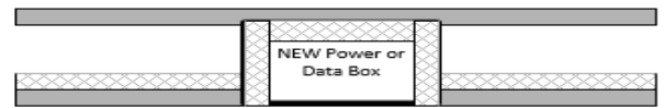
Option 2: worker to install new power utility wall box – box is lead Lined by manufacturer
