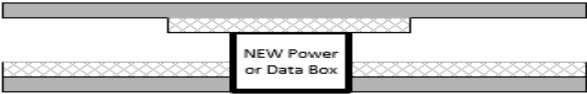
Option 1: worker to install new power utility wall box and add Lead Lining to wall behind box If worker can access posterior wall entry
