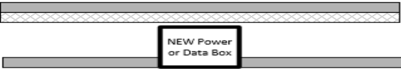
Option 3: worker to install new power utility wall box - no additional lead lining required if installation does not disrupt the existing shielding
