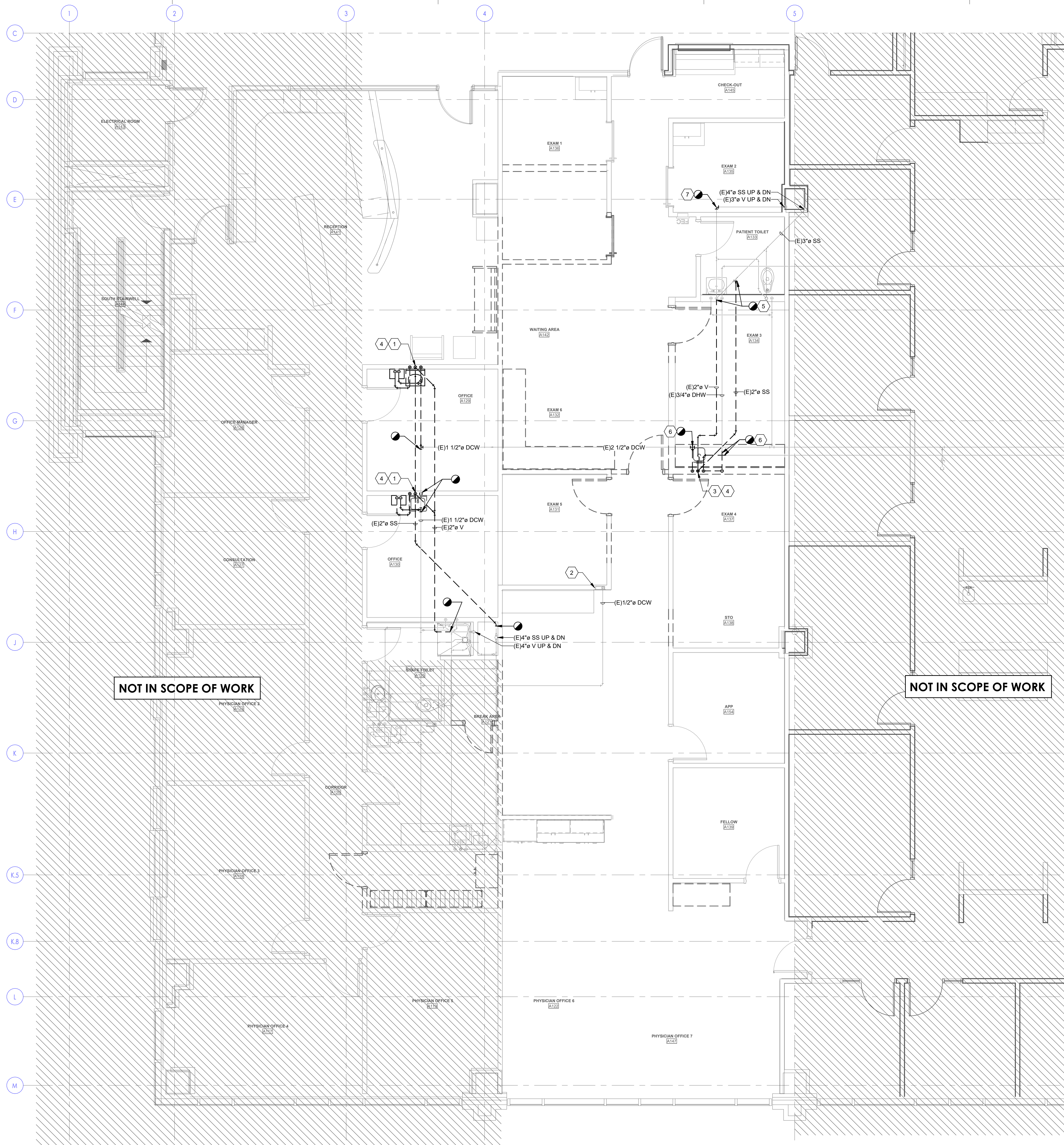
1 PLUMBING DEMOLITION PLAN - LEVEL 6 SCALE: 1/4" = 1'-0"
