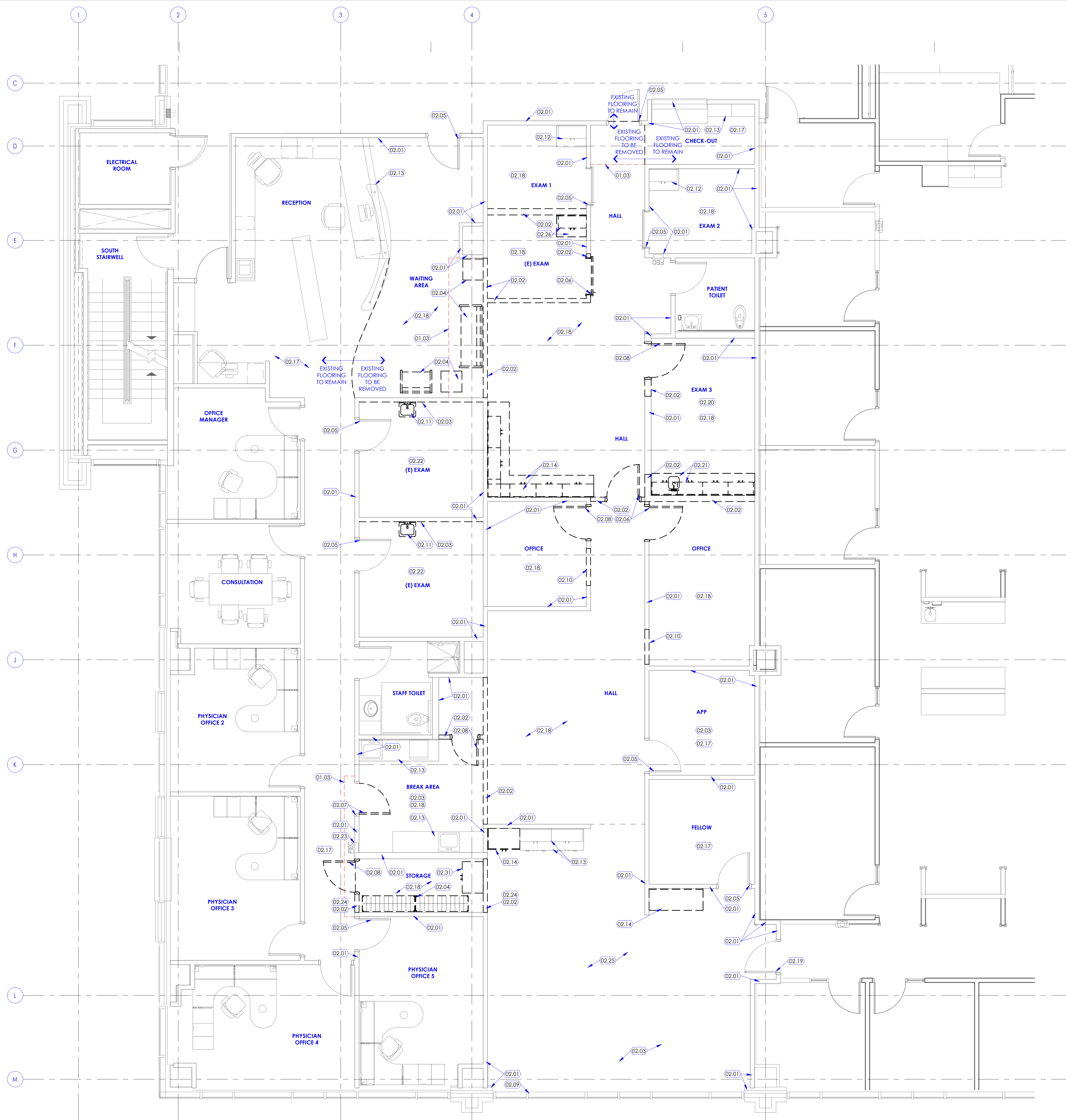
1 Demolition Floor Plan - Level 6 SCALE: 1/4" = 1'-0"
