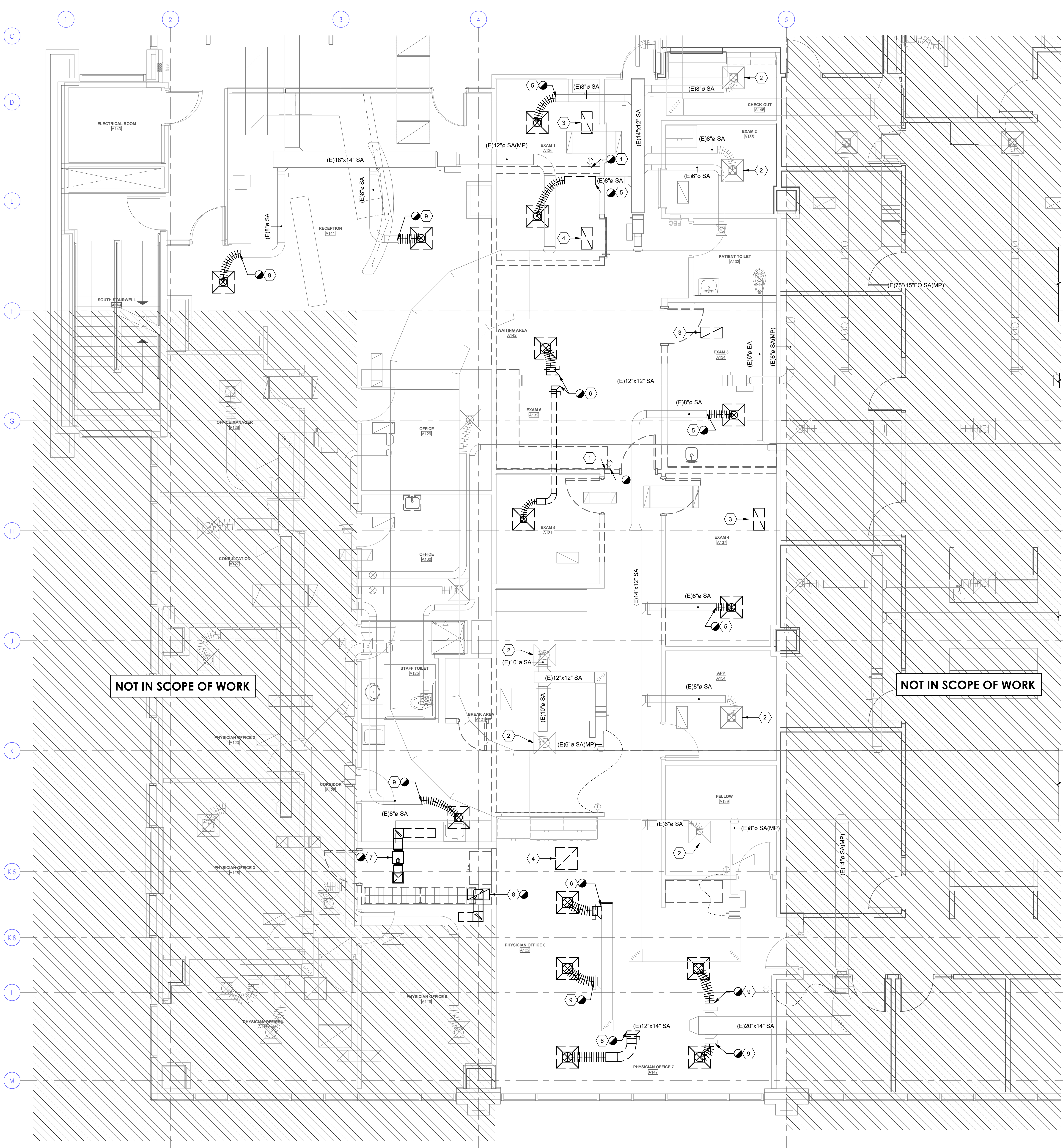
1 MECHANICAL DEMOLITION PLAN - LEVEL 6 SCALE: 1/4" = 1'-0"
