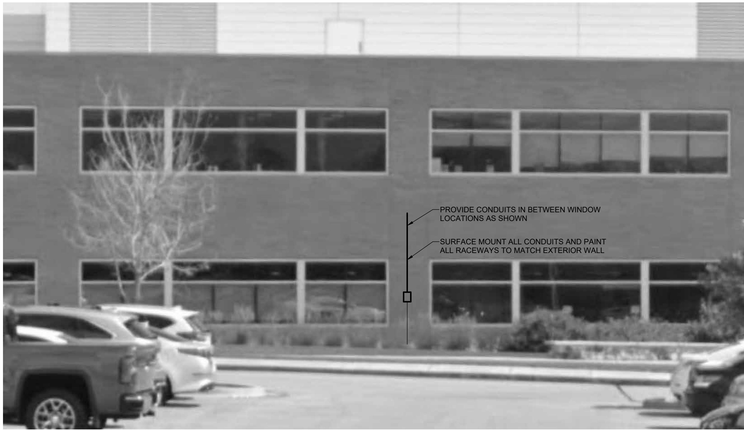
D4 TYPICAL RACEWAY EXTERIOR MOUNTING DETAIL SCALE: NTS
