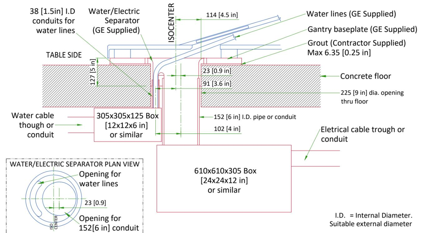
NOTE: PIPE, JUNCTION BOX, AND DUCT OR CONDUIT ARE TO BE SUPPLIED AND INSTALLED BY CUSTOMER OR CUSTOMER'S CONTRACTOR
