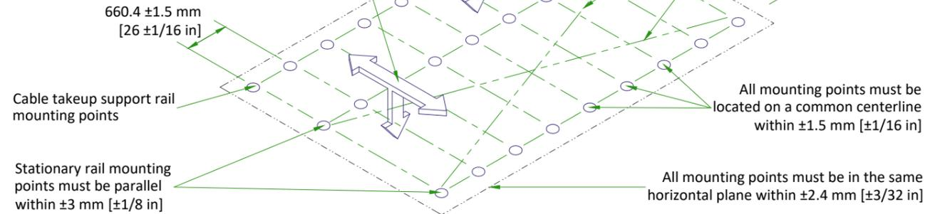
Each stationary rail must be mounted by bolts supplied or by 12 mm [1/2 in] as metric bolts. The maximum load per bolt must not exceed 1557 N [350 lbs] and each mounting bolt must not "PULL OUT" or otherwise fail under a vertically downward dead load of 6228 N [1400 lbs].
