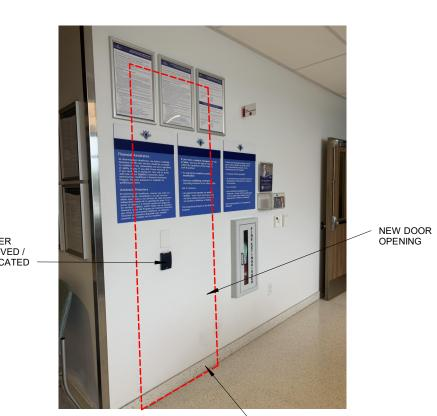
REMOVE TERAZZO BASE AS NECESSARY -SALVAGE FOR RE-INSTALLATION
