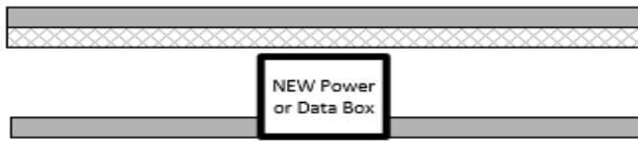
Option 3: worker to install new power utility wall box - no additional lead lining required if installation does not disrupt the existing shielding
