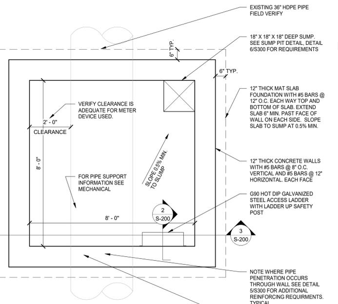
**2 METERING VAULT FOUNDATION PLAN VIEW**
