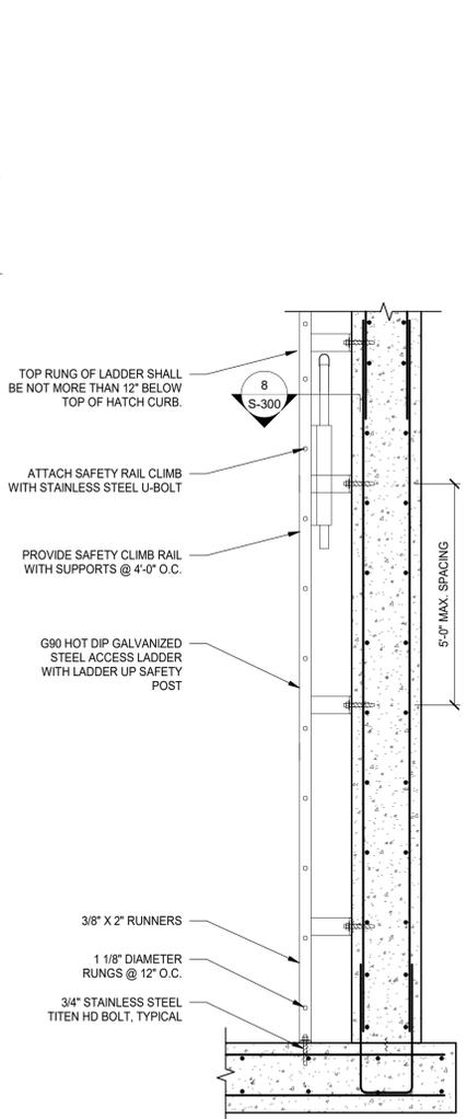
TOP RUNG OF LADDER SHALL BE NOT MORE THAN 12" BELOW TOP OF HATCH CURB.
