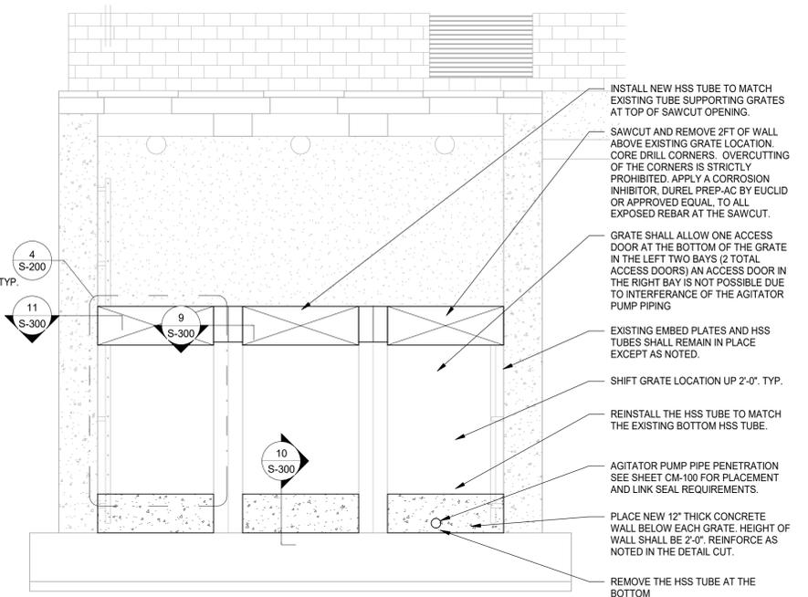
INSTALL NEW HSS TUBE TO MATCH EXISTING TUBE SUPPORTING GRATES AT TOP OF SAWCUT OPENING.
