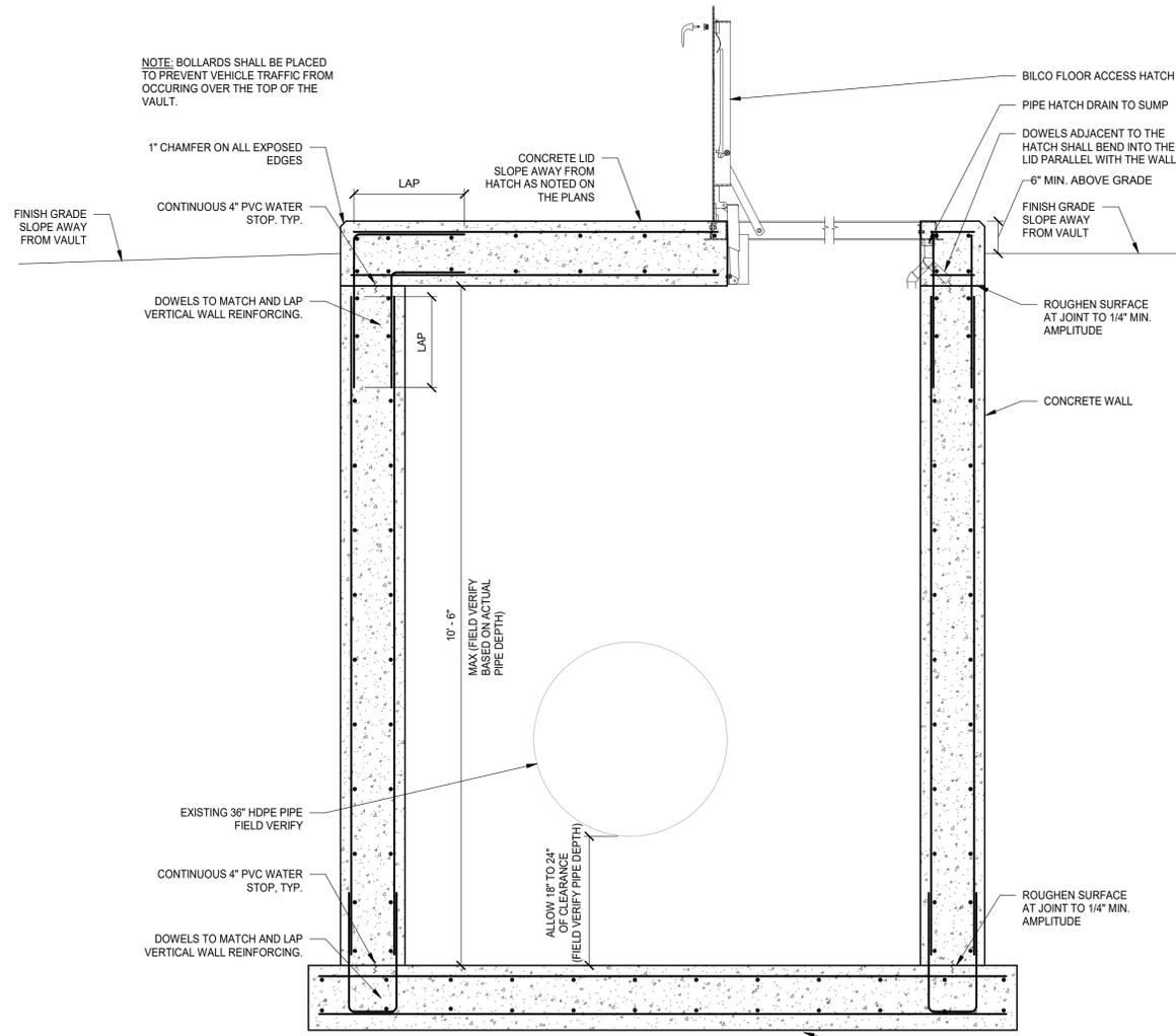
NOTE: BOLLARDS SHALL BE PLACED TO PREVENT VEHICLE TRAFFIC FROM OCCURRING OVER THE TOP OF THE VAULT.
