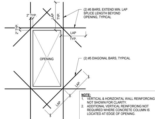
**5 TYP. ADD REINF @ OPENING IN CONCRETE WALL**
