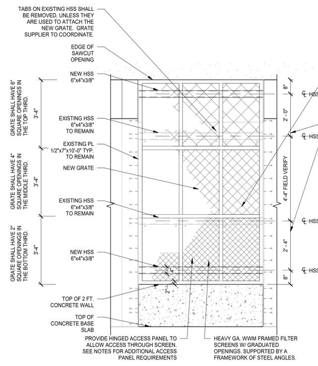
TABS ON EXISTING HSS SHALL BE REMOVED, UNLESS THEY ARE USED TO ATTACH THE NEW GRATE. GRATE SUPPLIER TO COORDINATE.
