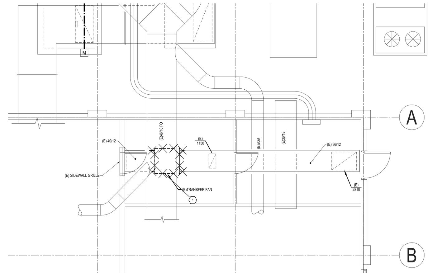
1 MECHANICAL DEMOLITION PLAN
