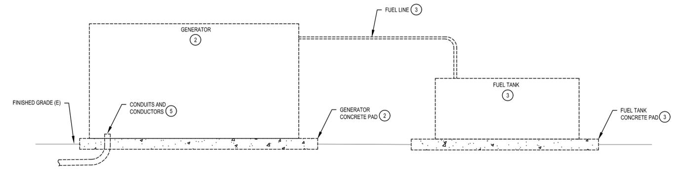
**3 GENERATOR AND FUEL TANK DEMOLITION ELEVATION DETAIL**
