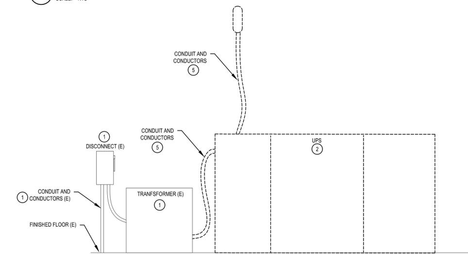
**2 UPS DEMOLITION ELEVATION DETAIL**
