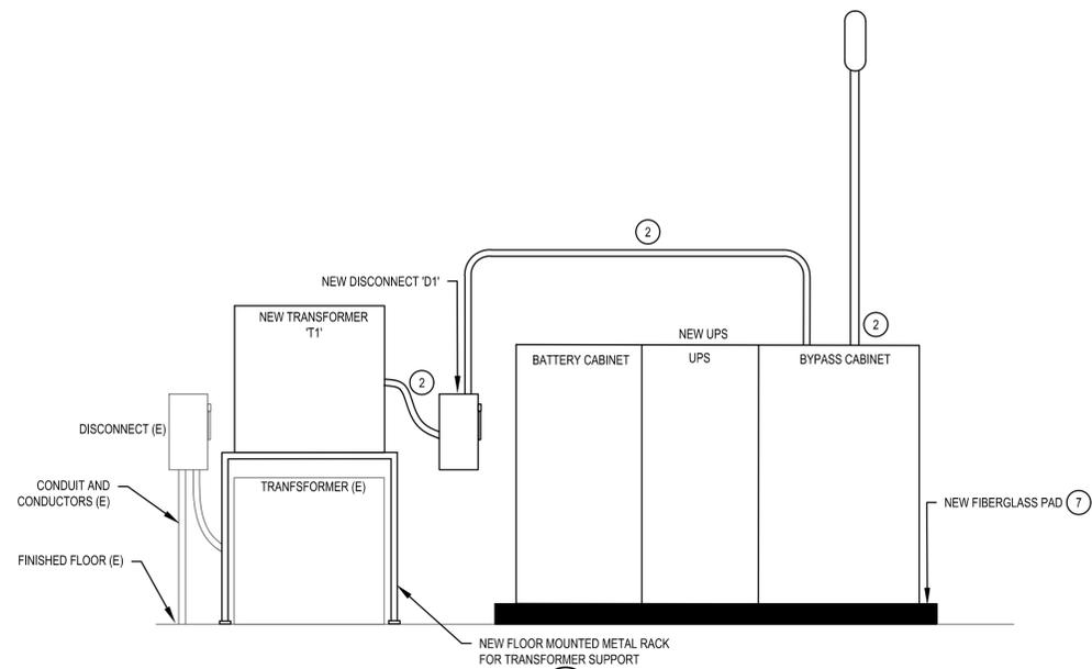
**2 NEW UPS ELEVATION DETAIL**
