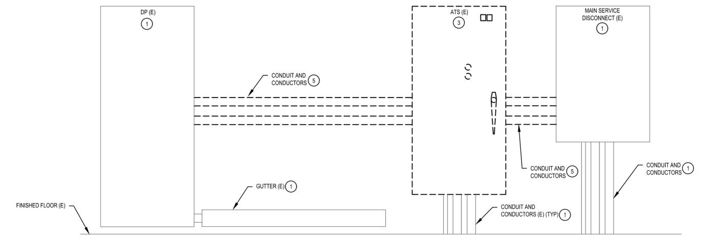
**3 ATS DEMOLITION ELEVATION DETAIL**
