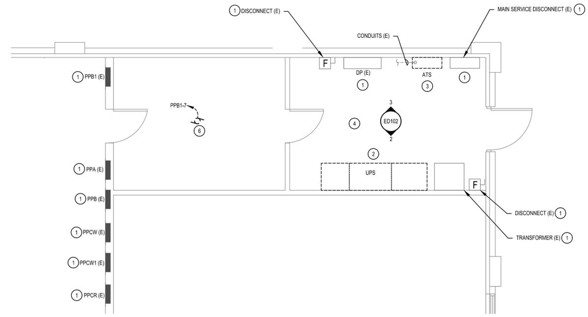
**1 DEMOLITION FLOOR PLAN**
