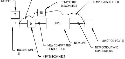
DISCONNECT EXISTING PERMANENT FEEDERS. CONNECT TEMPORARY GENERATOR AND ATS TO BUILDING ELECTRICAL SYSTEM. DEMOLISH EXISTING ATS, GENERATOR, FUEL TANK, AND ASSOCIATED CONDUITS, FUEL LINES , CONDUCTORS AS SHOWN. POWER OUTAGE IS EXPECTED DURING THIS STEP. COORDINATE POWER OUTAGE TIME WITH OWNER PRIOR T
