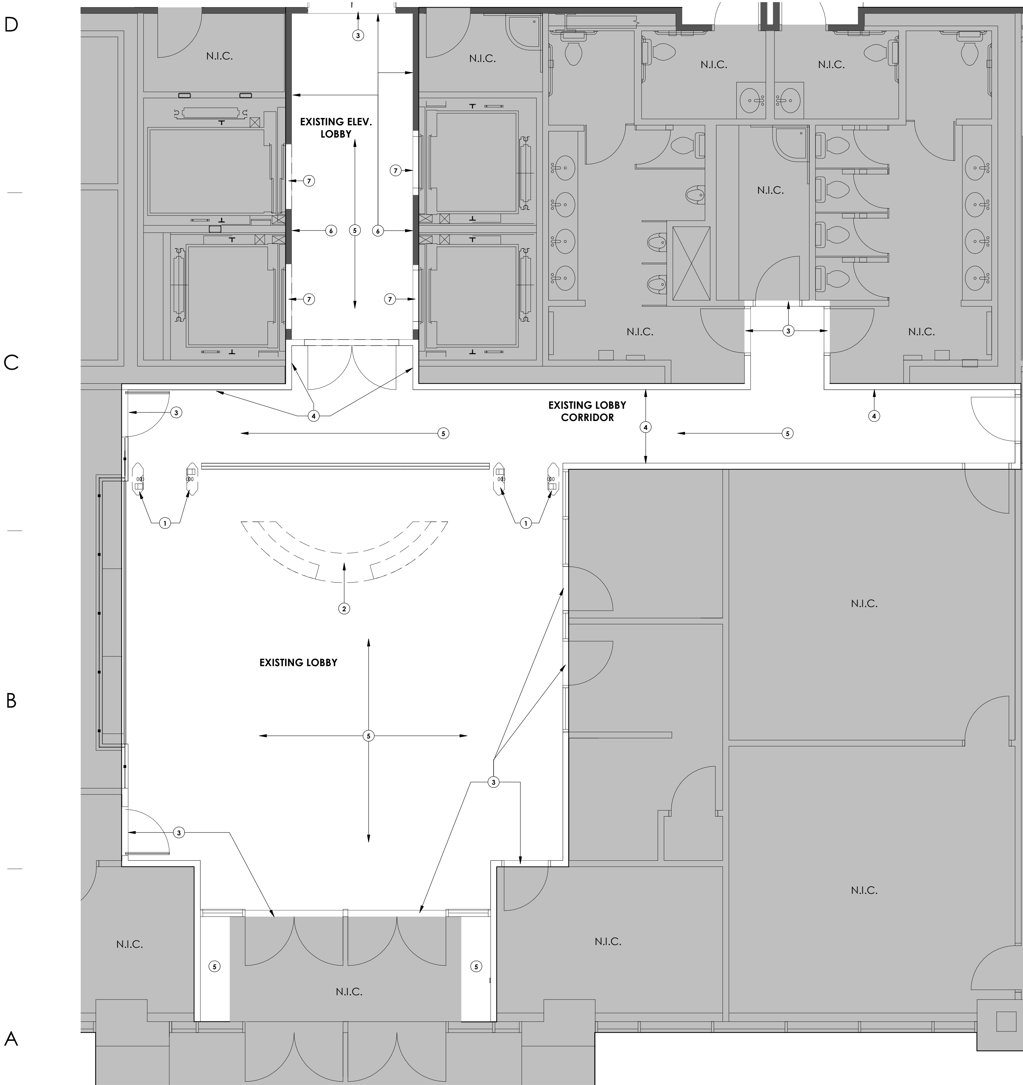
A1 DEMO FLOOR PLAN - LEVEL 01 LOBBY & ELEVATOR LOBBY 1/4" = 1'-0", DWG REF: A010
