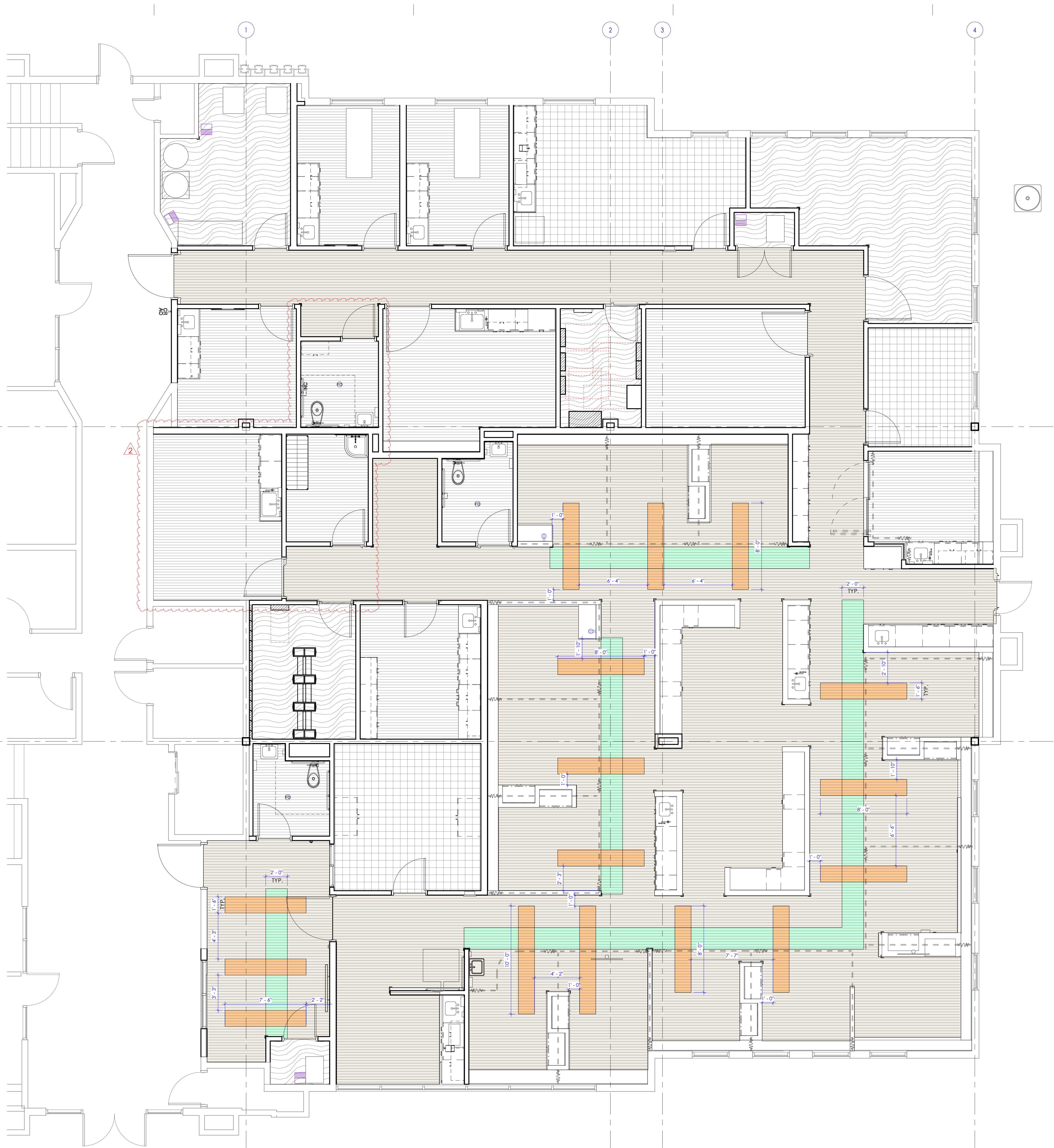
1 Floor Pattern Plan Level 1 SCALE: 1/4" = 1'-0"
