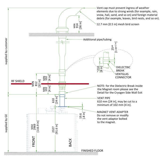
Waveguide is contractor supplied. Minimum 812 mm [32 in]. Must extend at least 100 mm [4 in] on magnet room side of the wall/ceiling and 25±6 mm [1±0.25 in] from the GE supplied pipe below isolation joint. Magnet room end must not be more than 2969 mm [117 in]above finished floor.
