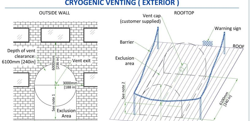
(1) Restricted area: minimum distance between vent pipe and ground is 3660mm [144 in]. Barriers are required. Public area: barriers are not required if height is > 5000mm [197 in].
