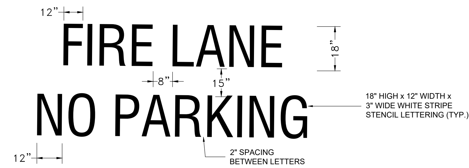
6 FIRE LANE NO PARKING PAVEMENT MARKING Scale: (NOT TO SCALE)
