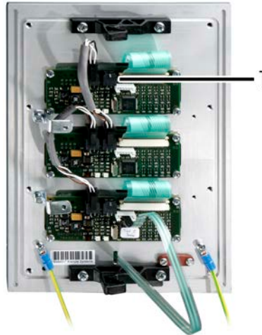
Figure 19. SK enclosure integrated wall control unit with keypad, interior
