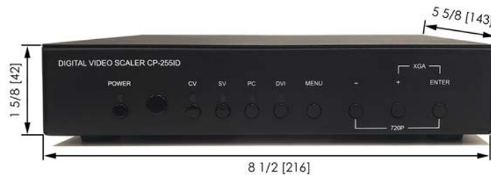
Figure 10. Front View Converter Box (dimensions are in inches [mm])
